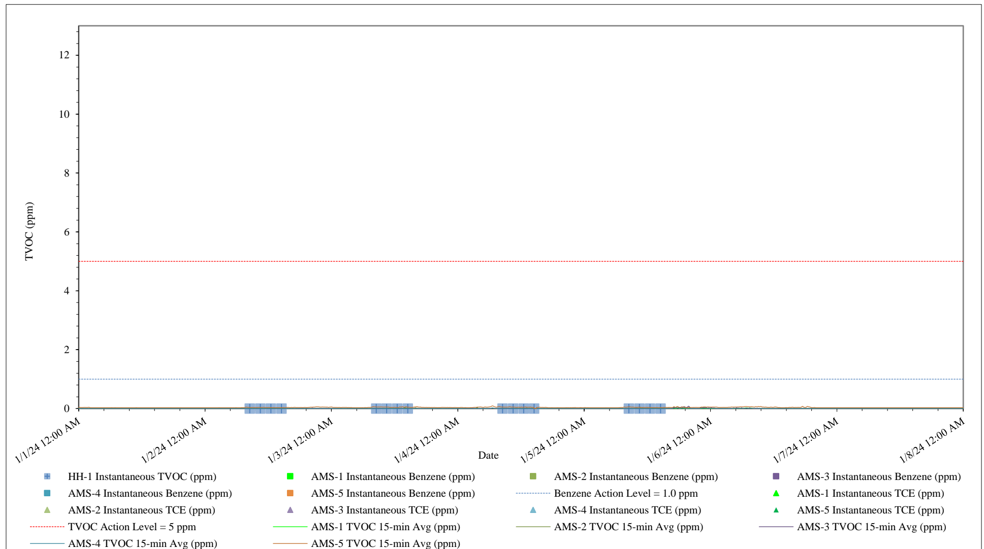
Figure 2 – Summary of TVOC, Benzene, and Tri-chloroethylene Concentrations 01/01/24 through 01/07/24
