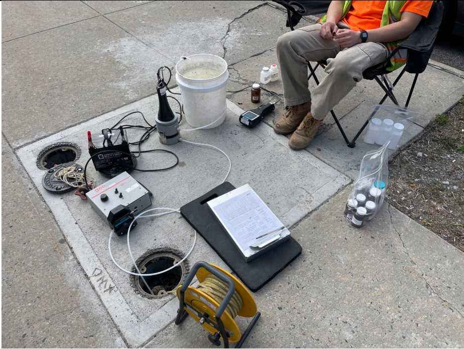
Photo 3: Looking southeast, view of Roux collecting groundwater from sentinel well SW-02S.
