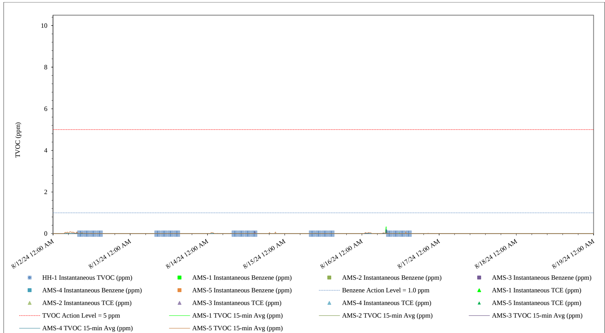
Figure 2 – Summary of TVOC, Benzene, and Tri-chloroethylene Concentrations 08/12/24 through 08/18/24
