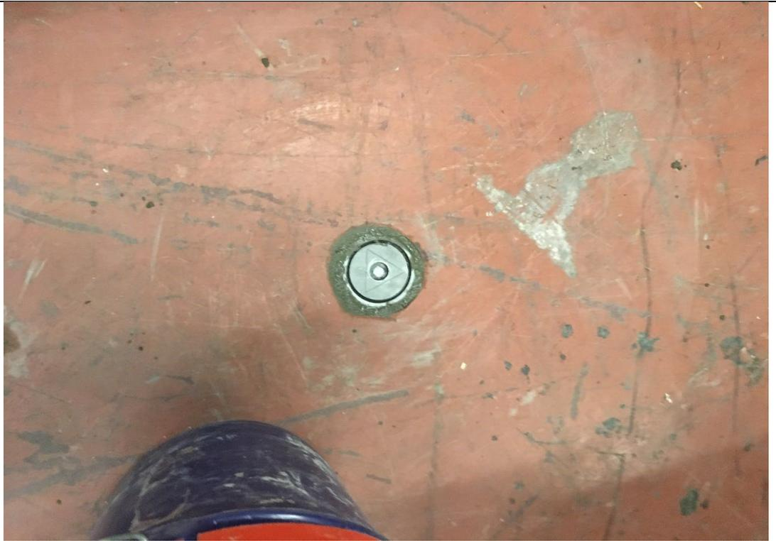
Photo 2. Sub-slab soil vapor sample in process in Facilities Building.
