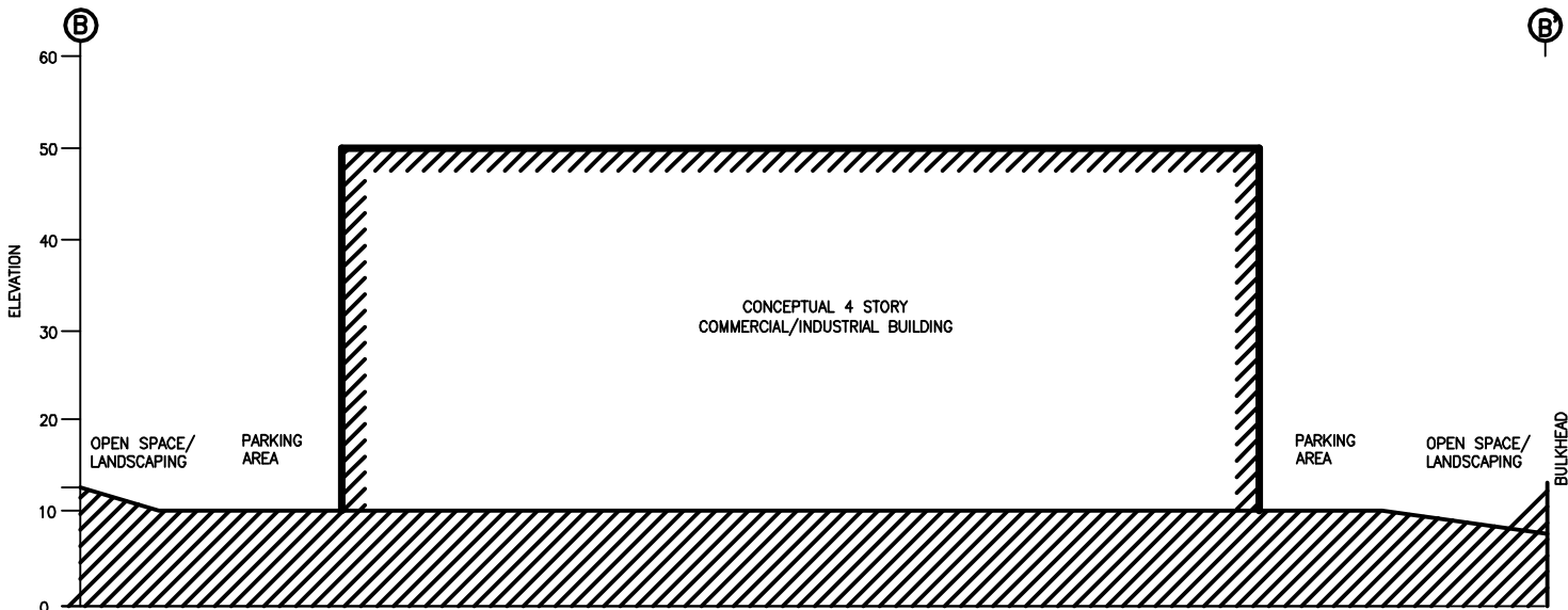
CONCEPTUAL SITE PROFILE CROSS SECTION B-B' HORIZONTAL 1"=60' VERTICAL 1"=10'
