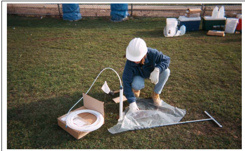
Photo/Frame No.: 6 Direction of View: Northeast Date/Time: 3-14-00/07:55 Subject: Preparation of soil gas probe at SG-1. Photographer: R. Watt
