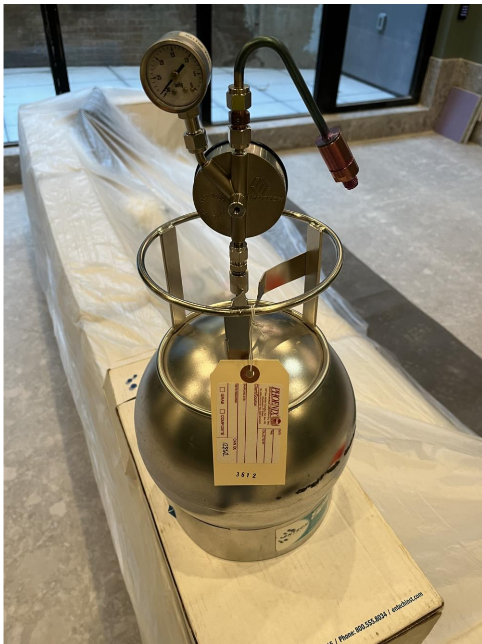
IA-3 Duplicate starting sampling pressure of 29 inHg.
