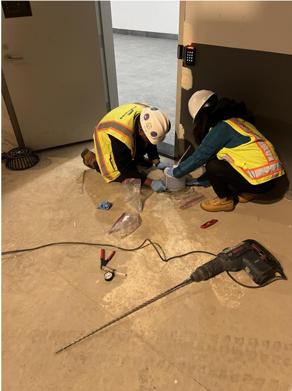
Creating an bentonite seal around the bucket.
