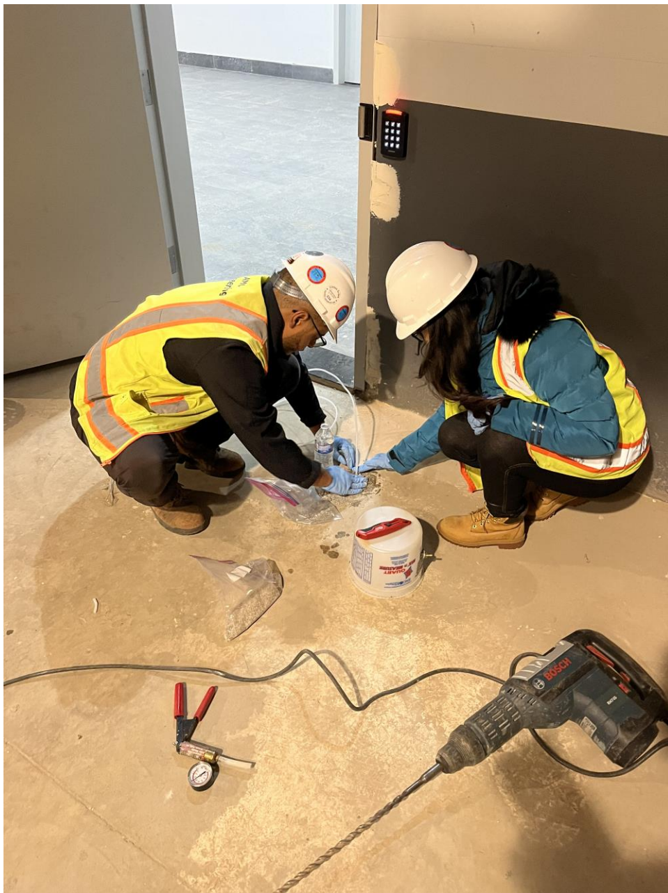
Creating an Bentonite seal around the test tube. SS-2 location.
