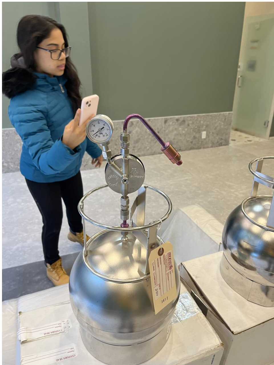
IA-3 starting sampling pressure of 27.5 inHg.
