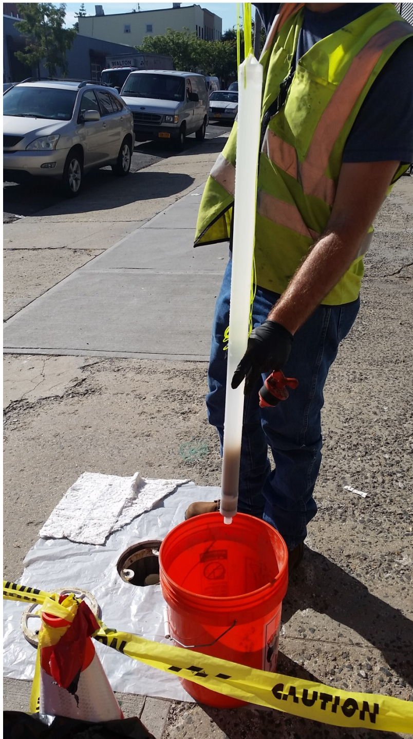
Photo 11: 9/16/15: Bailer showing DNAPL at DEC-136D
