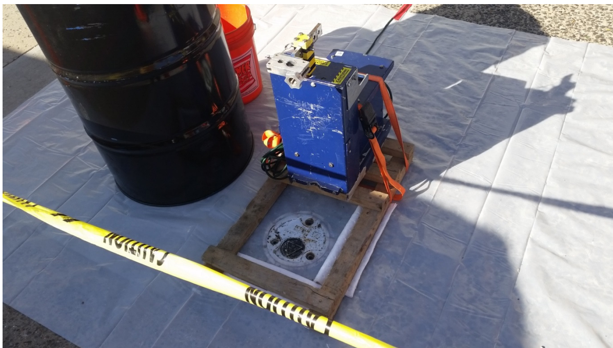
Photo 8: 9/15/15: Waterra pump set up for DNAPL removal at DEC-136
