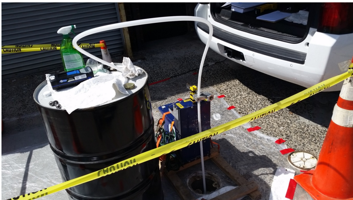
Photo 6: 9/14/15: Watterra pump and drum set up for DNAPL removal at DEC-136
