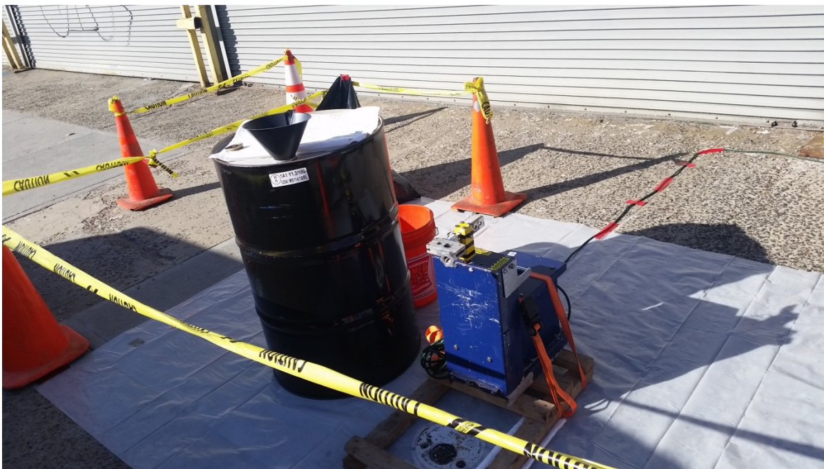
Photo 9: 9/15/15: Waterra pump and drum set up for DNAPL removal at DEC-136
