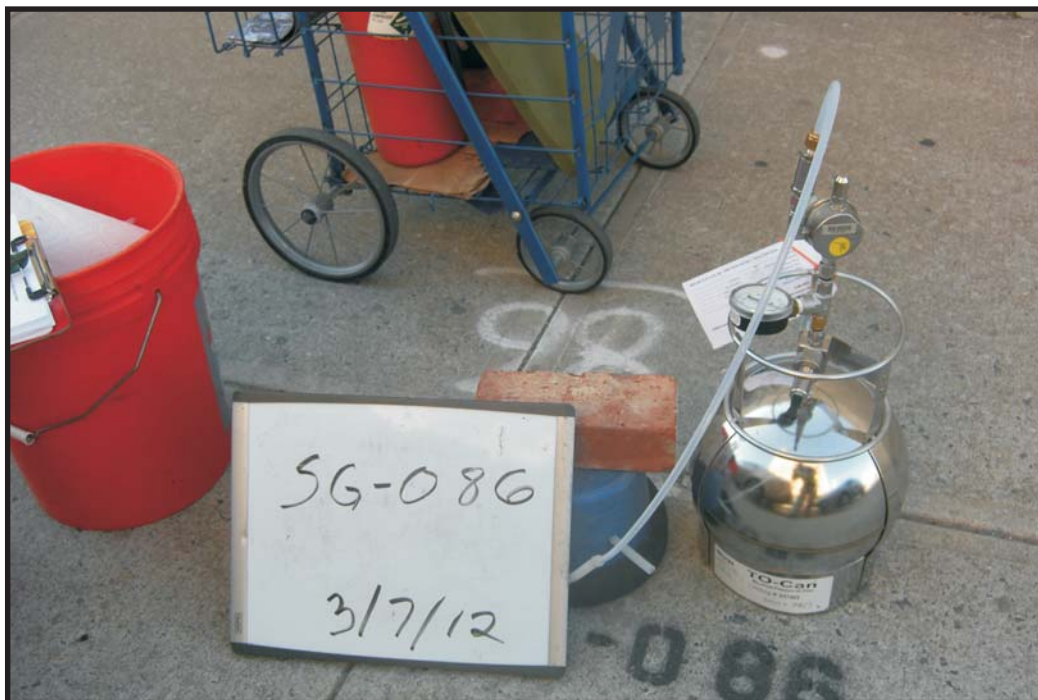
3/7/12: Soil-gas sample collection at SG-086.
