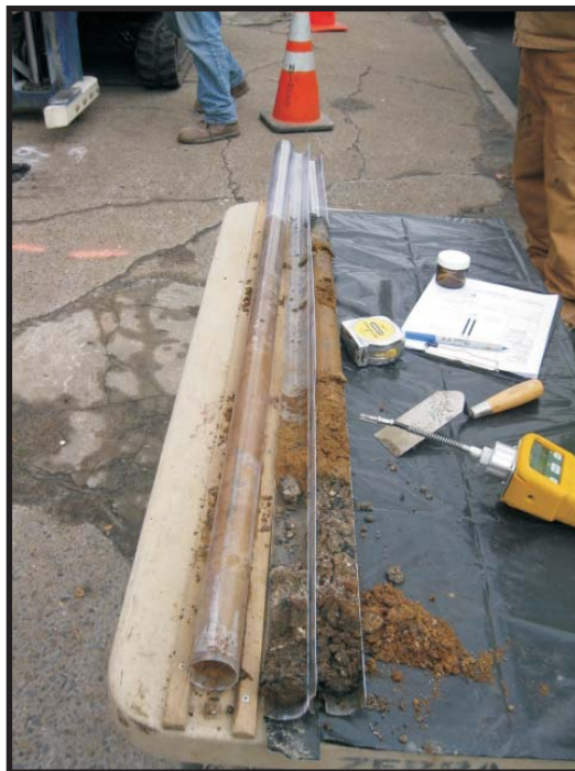
3/1/12: Photograph of Macro core sample collected from SG-119.
