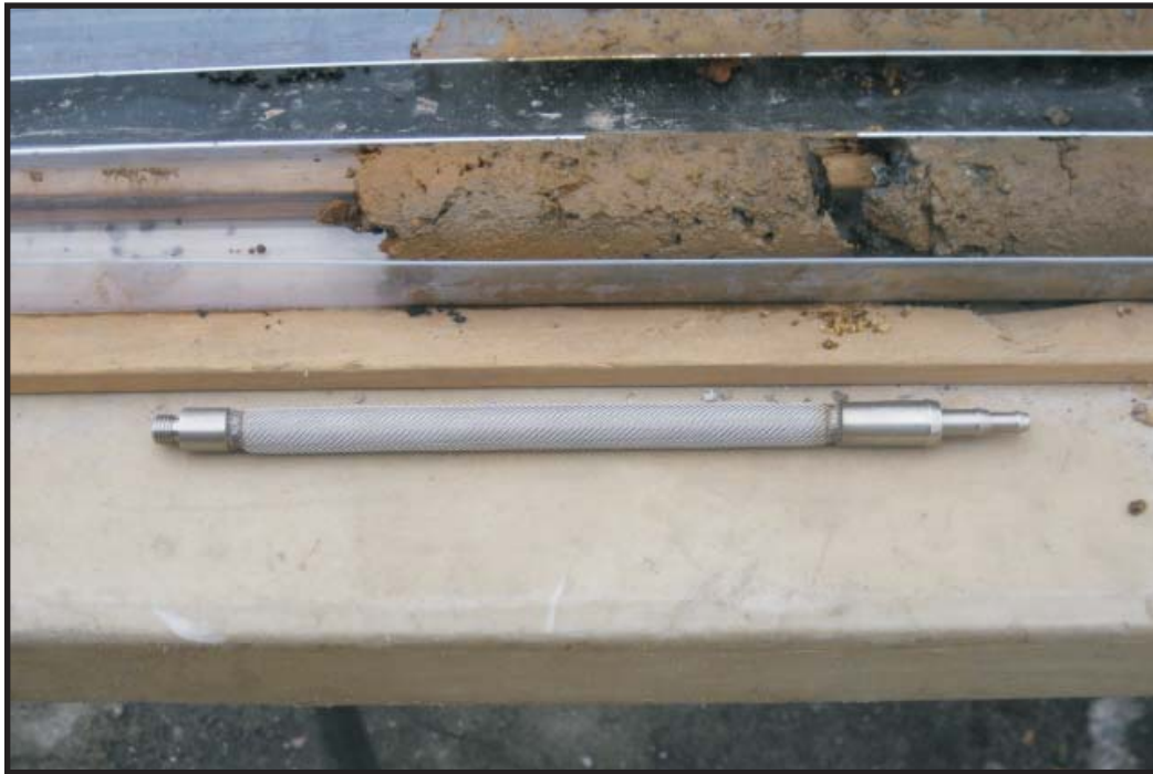
3/1/12: Photograph of 6-inch long soil-gas implant prior to installation.
