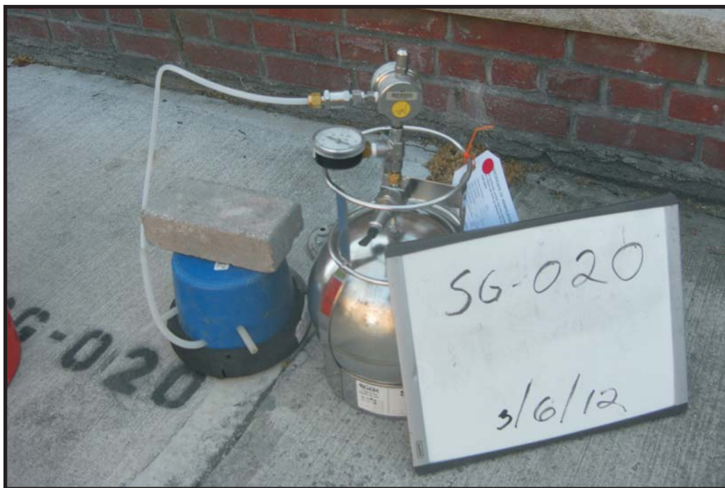
3/6/12: Soil-gas sample collection at SG-020.
