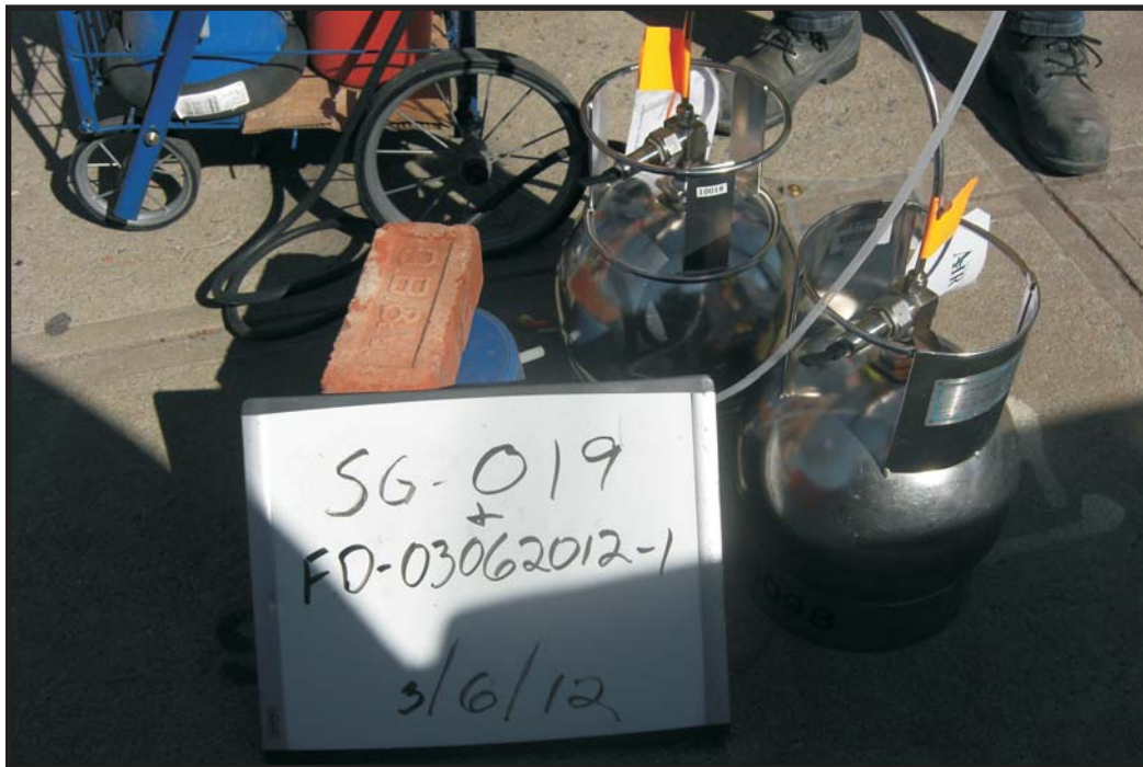
3/6/12: Soil-gas sample collection at SG-019 and field duplicate FD-03062012-1.
