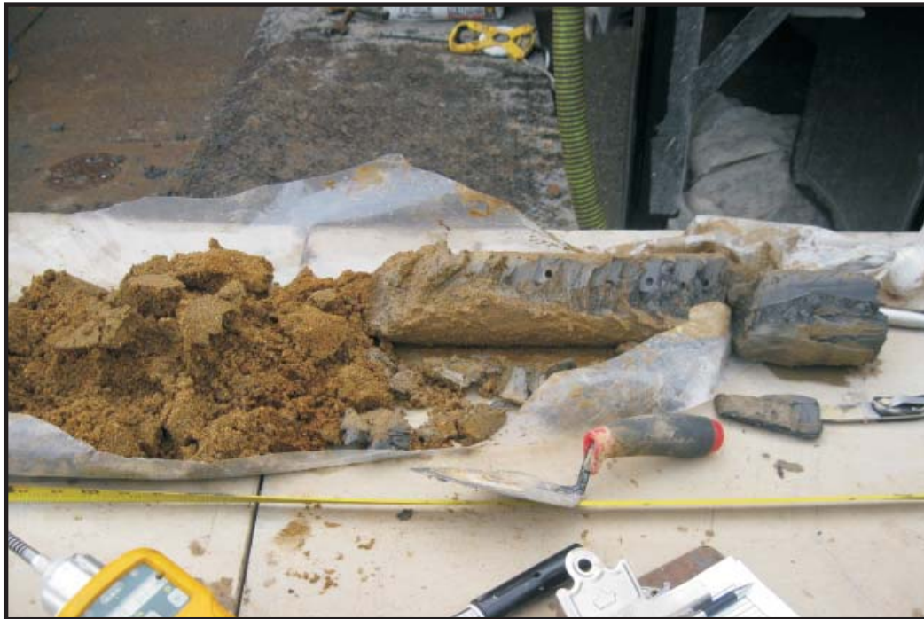
3/13/12: Interface of sand and gray lacustrine silty clay at 78.5 feet bgs in DEC-028D.
