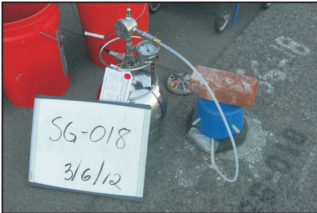
3/6/12: Soil-gas sample collection at SG-018.
