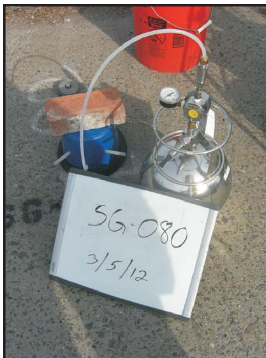
3/5/12: Soil-gas sample collection at SG-080.
