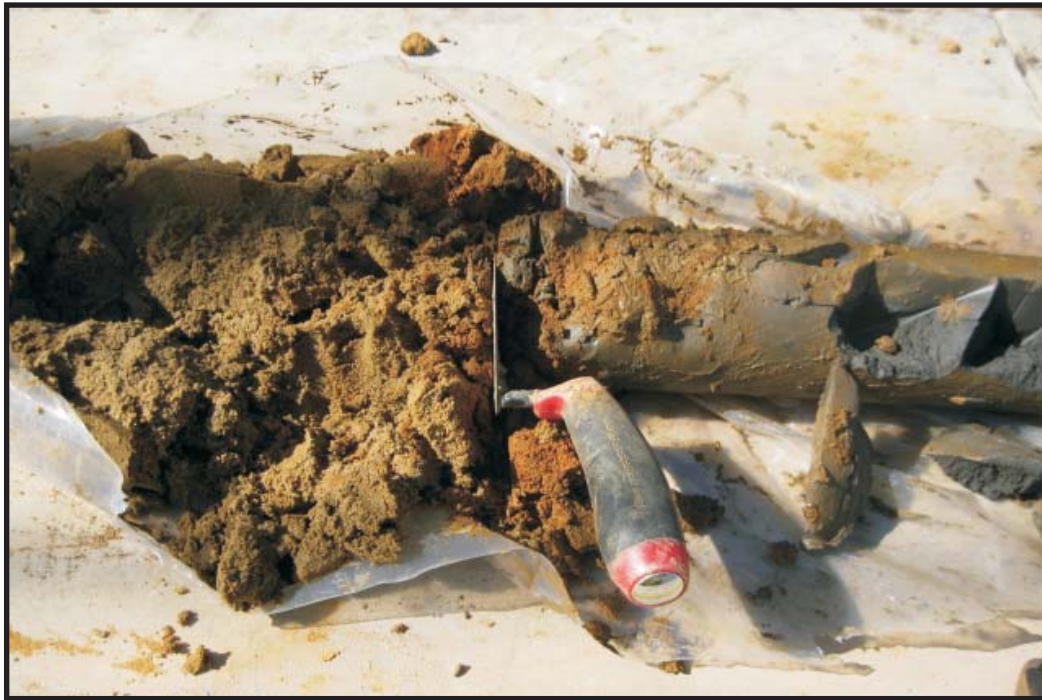
3/14/12: Interface of sand and gray lacustrine silty clay at 72 feet bgs in DEC-011D.
