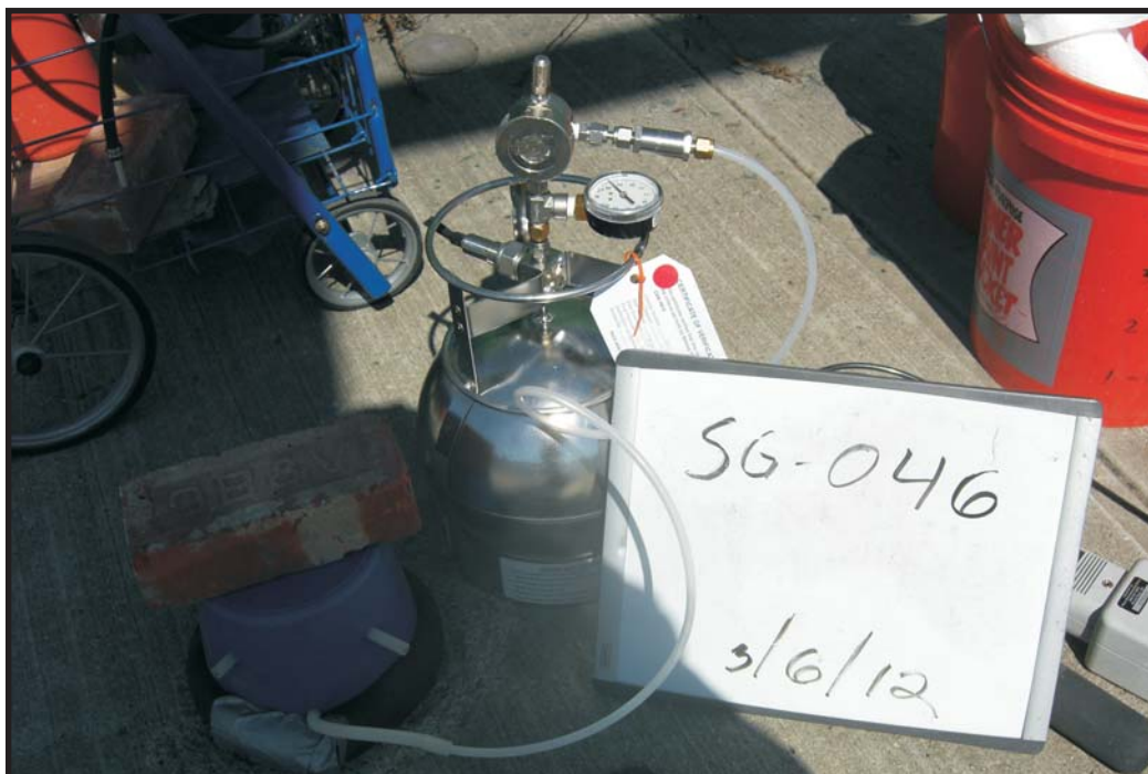
3/6/12: Soil-gas sample collection at SG-046.
