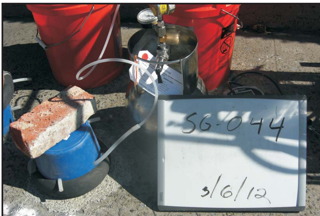
3/6/12: Soil-gas sample collection at SG-044.
