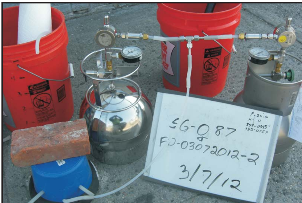
3/7/12: Soil-gas sample collection at SG-087 and field duplicate FD-03072012-2. Duplicate sample not used, summa can expired too quickly.
