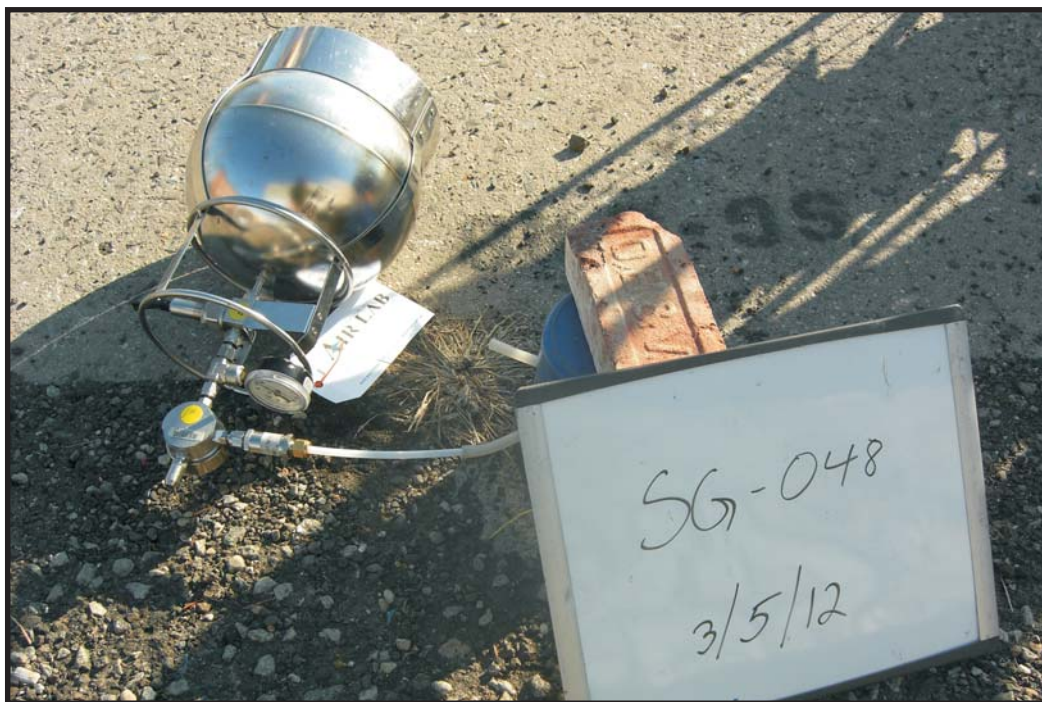
3/5/12: Soil-gas sample collection at SG-048.
