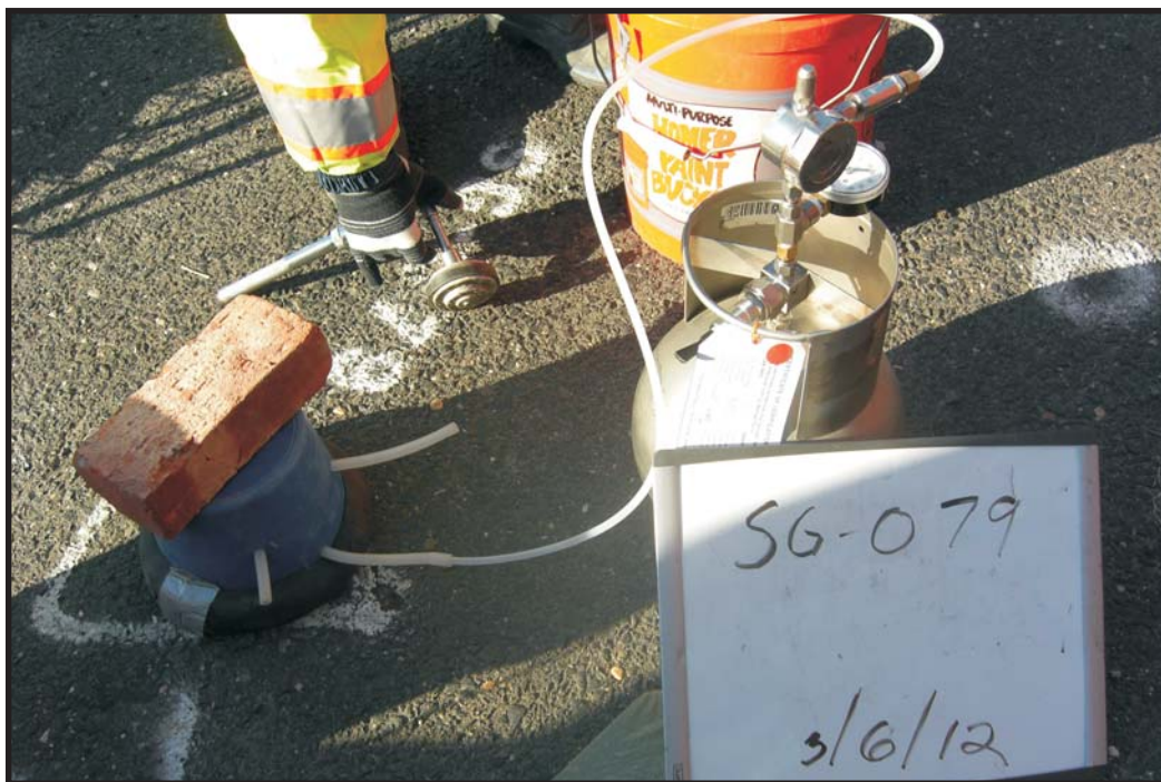
3/6/12: Soil-gas sample collection at SG-079.
