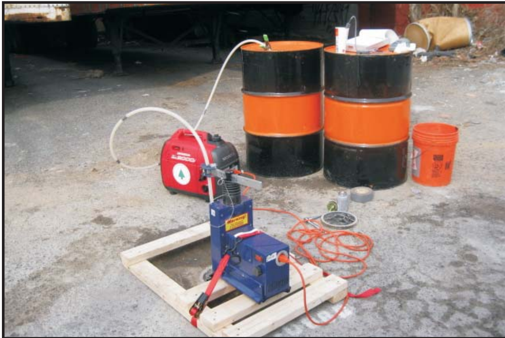
3/7/12: Well development at DEC-088D using Watterra Pump.
