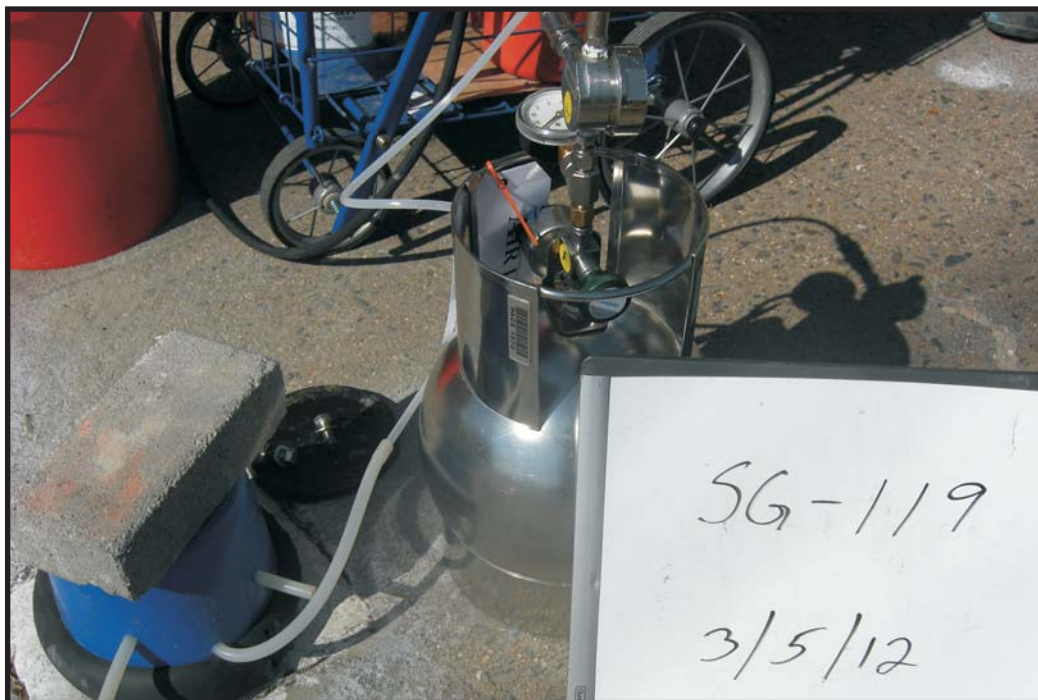
3/5/12: Soil-gas sample collection at SG-119.
