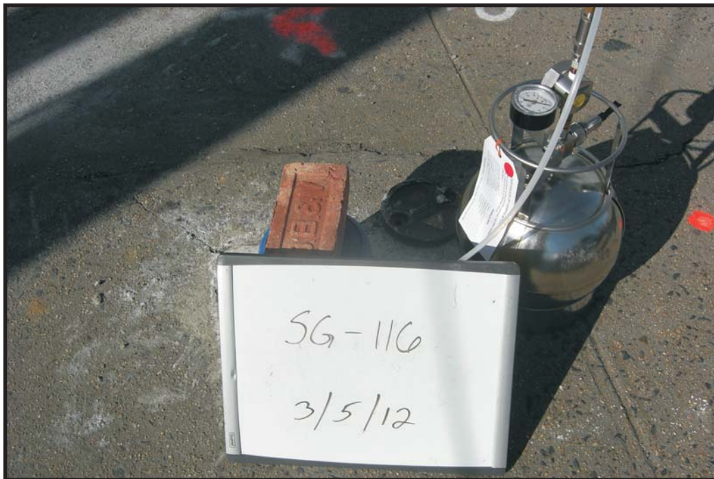
3/5/12: Soil-gas sample collection at SG-116.
