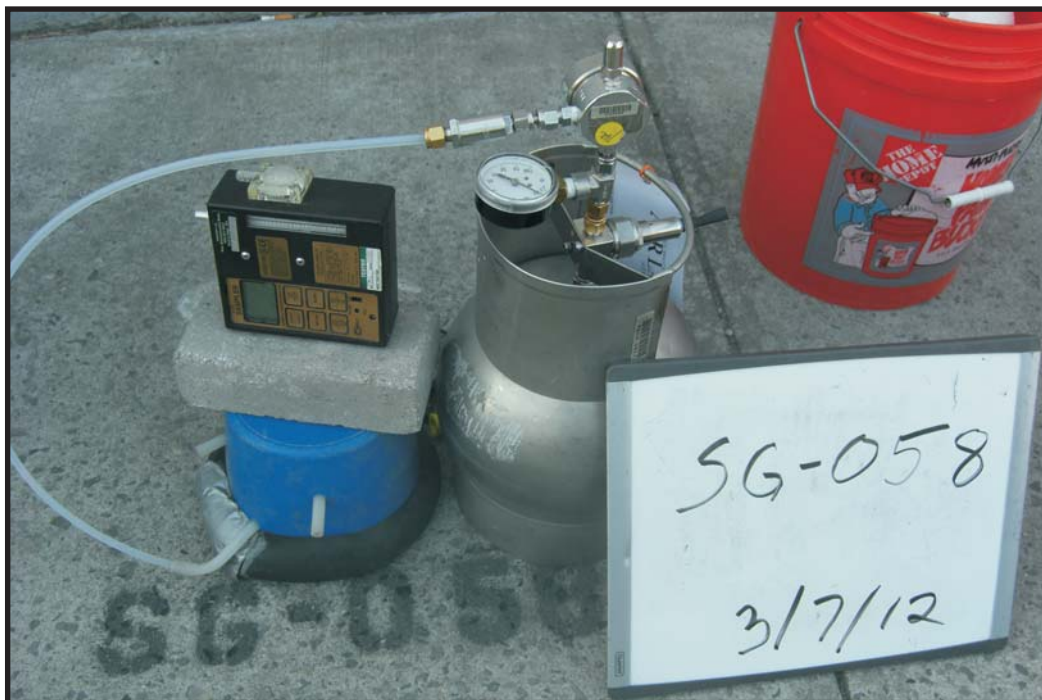
3/7/12: Soil-gas sample collection at SG-058.
