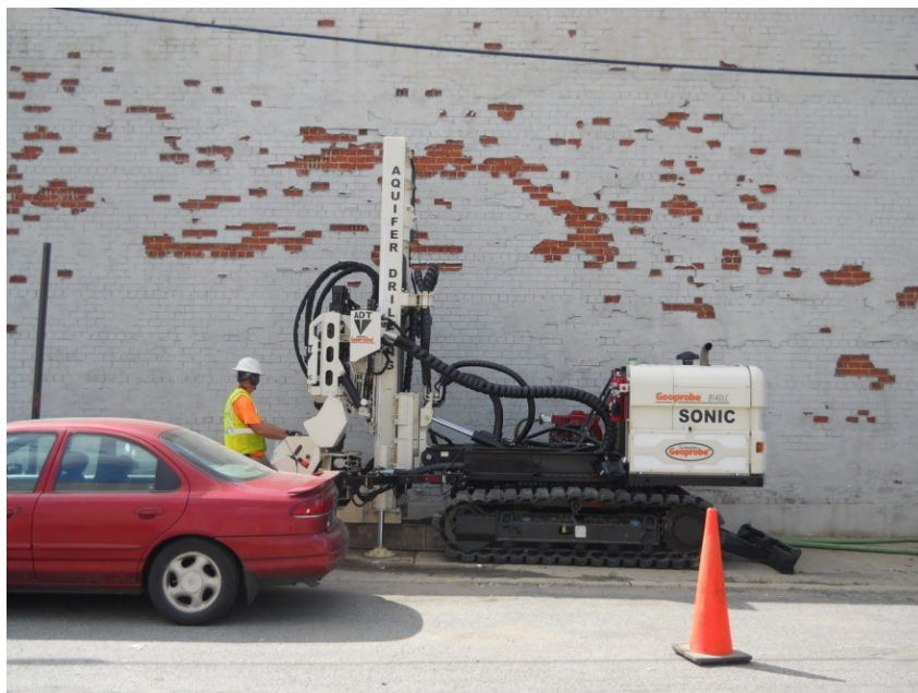
Photo 12: ADT Sonic Drill Rig.
