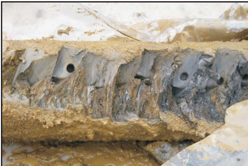
3/13/12: Close up photograph of gray lacustrine silty clay at DEC-028D.
