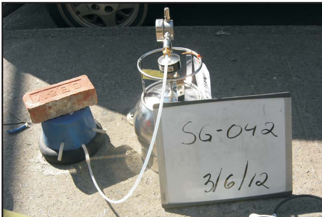
3/6/12: Soil-gas sample collection at SG-042.
