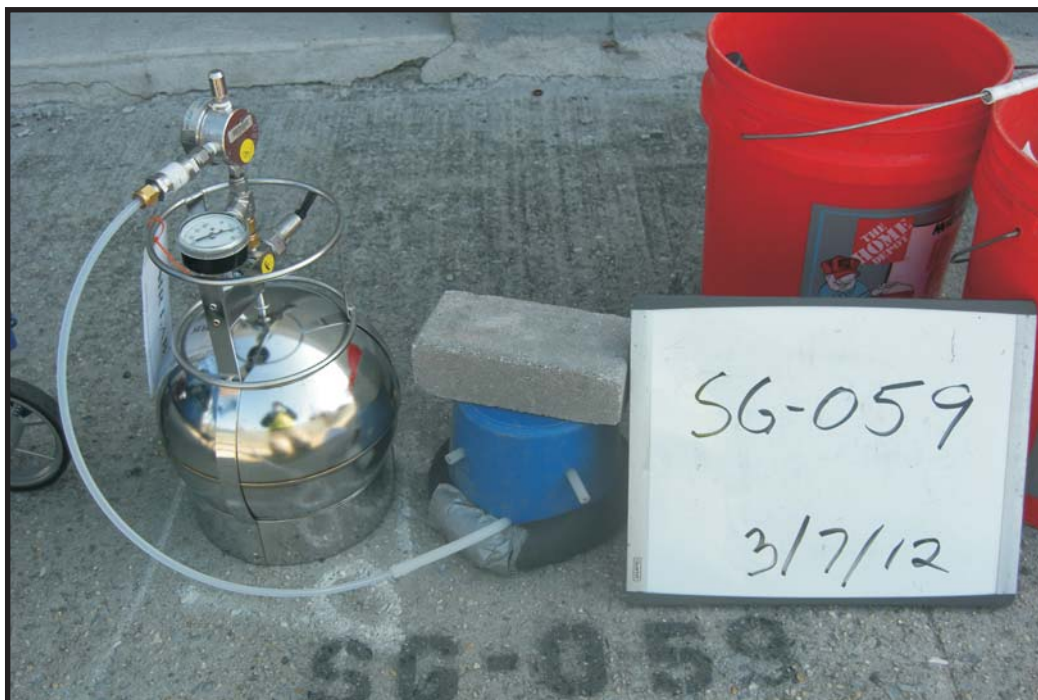
3/7/12: Soil-gas sample collection at SG-059.
