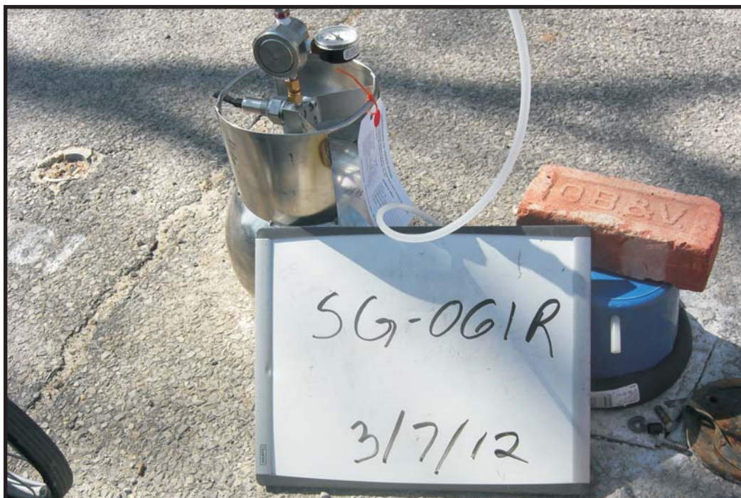
3/7/12: Soil-gas sample collection at SG-061R.
