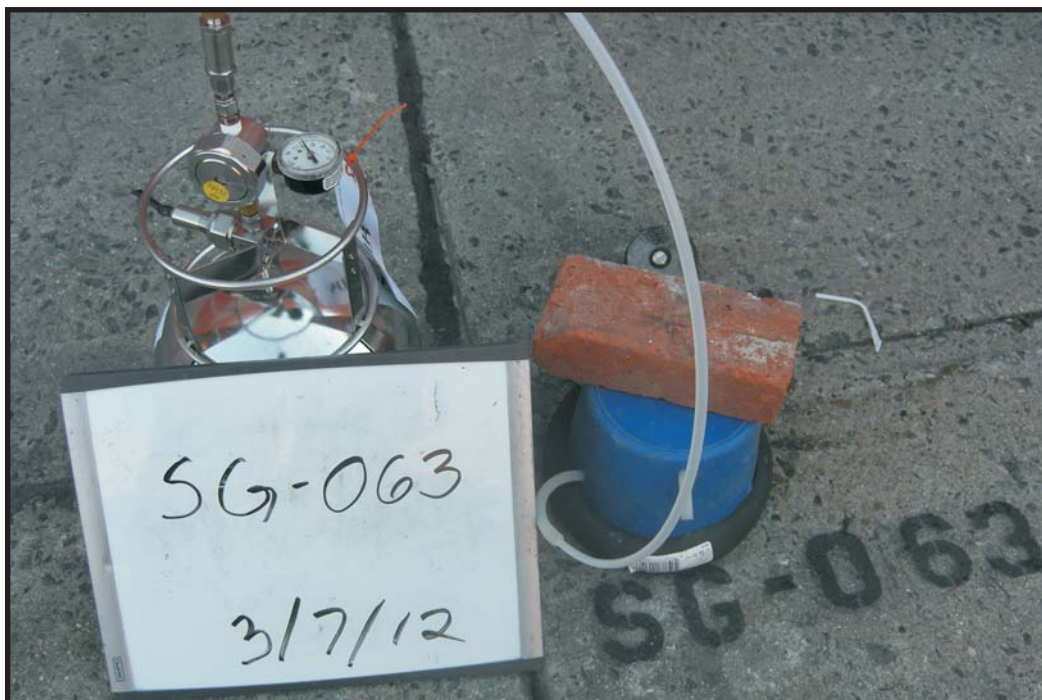
3/7/12: Soil-gas sample collection at SG-063.
