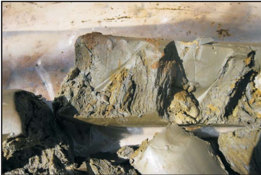
3/14/12: Close up photograph of gray lacustrine silty clay at DEC-011D.
