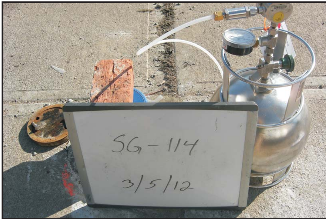
3/5/12 Soil-gas sample collection at SG-114.
