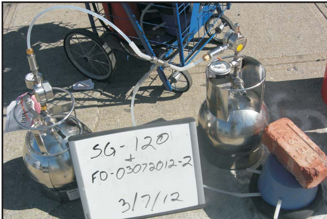
3/7/12: Soil-gas sample collection at SG-120 and field duplicate FD-03072012-2.
