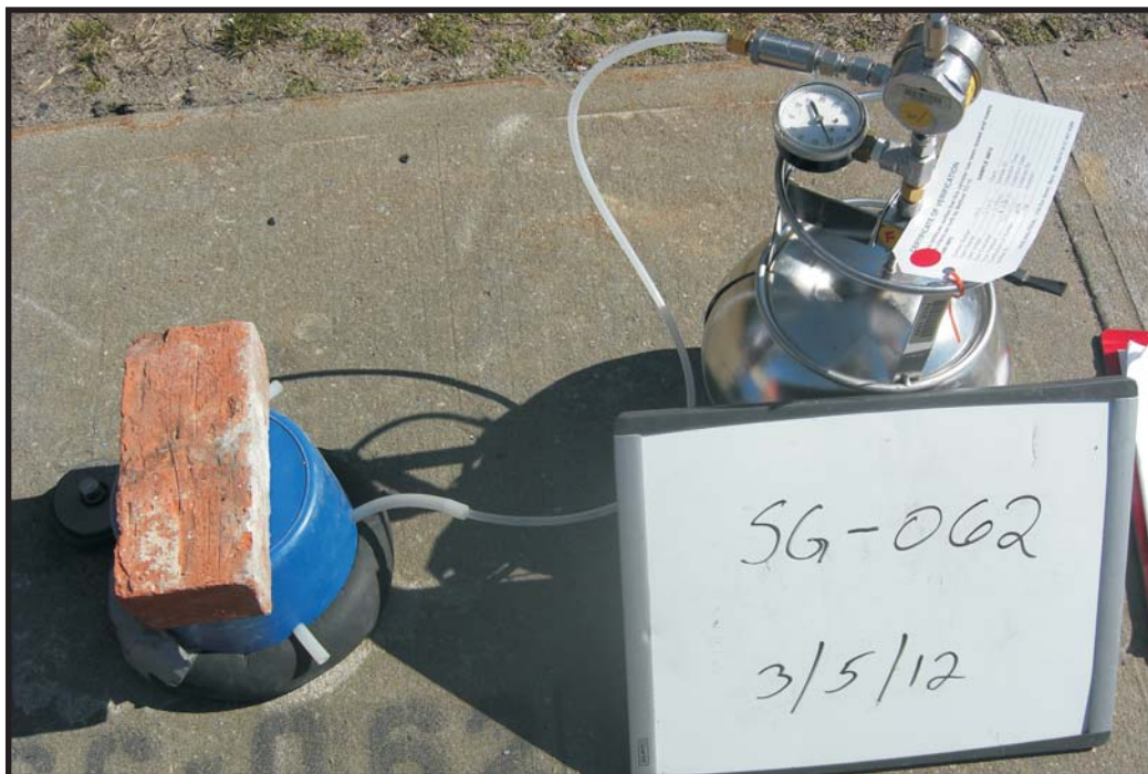
3/5/12: Soil-gas sample collection at SG-062.
