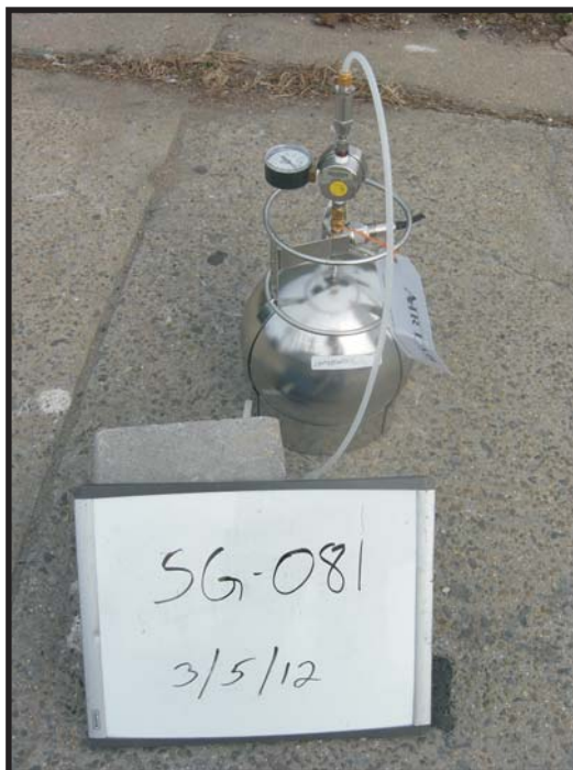
3/5/12: Soil-gas sample collection at SG-081.
