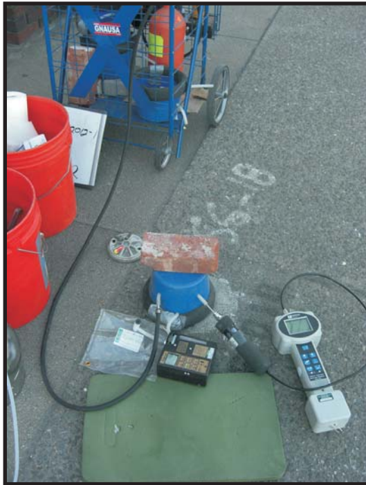
3/6/12: Example of helium testing at SG-018 prior to sample collection.
