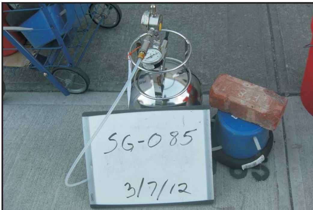
3/7/12: Soil-gas sample collection at SG-085.
