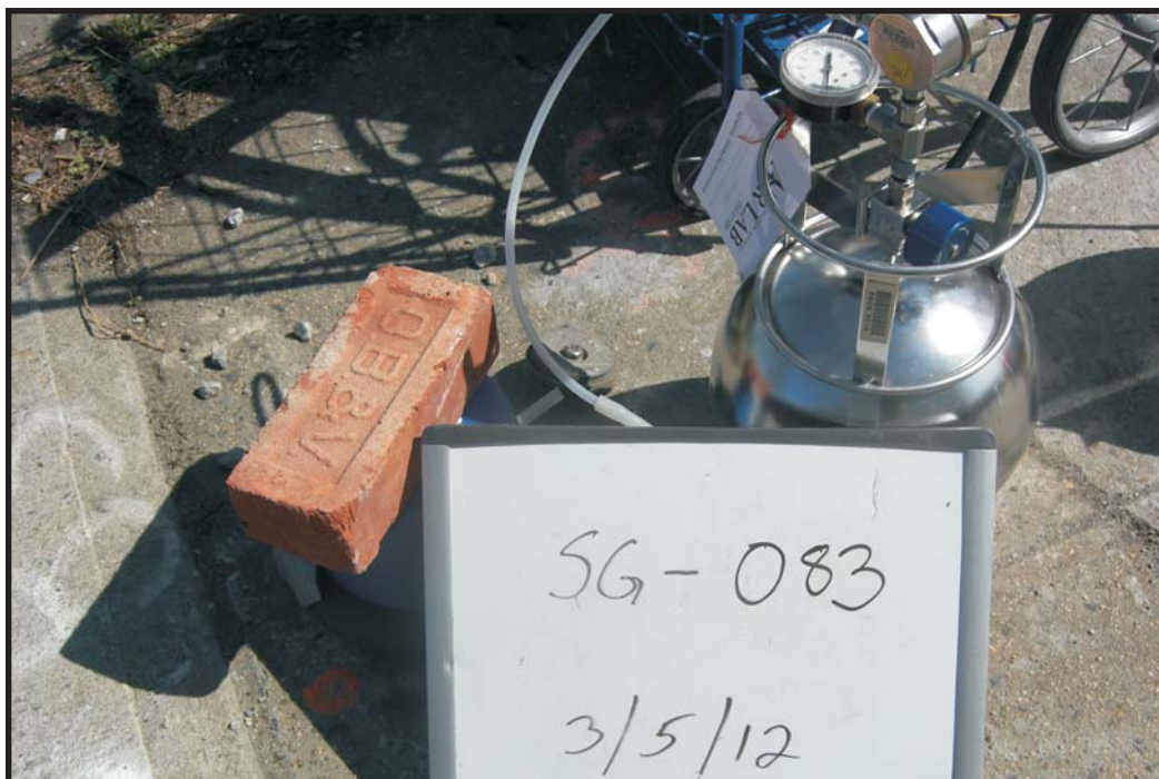
3/5/12: Soil-gas sample collection at SG-083.
