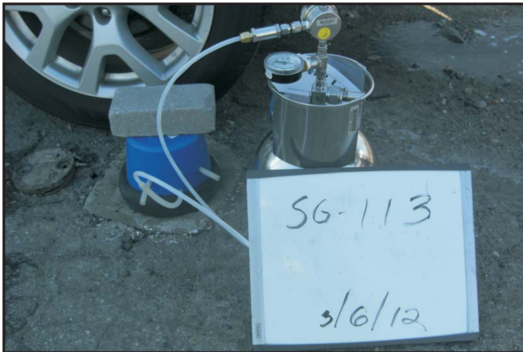
3/6/12: Soil-gas sample collection at SG-113.
