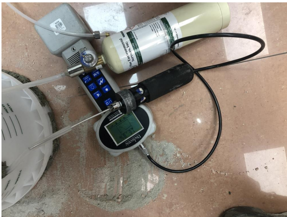
Photo 1: View of seal integrity testing on permanent sub-slab soil vapor point SSV-01 (12/12/2020)
