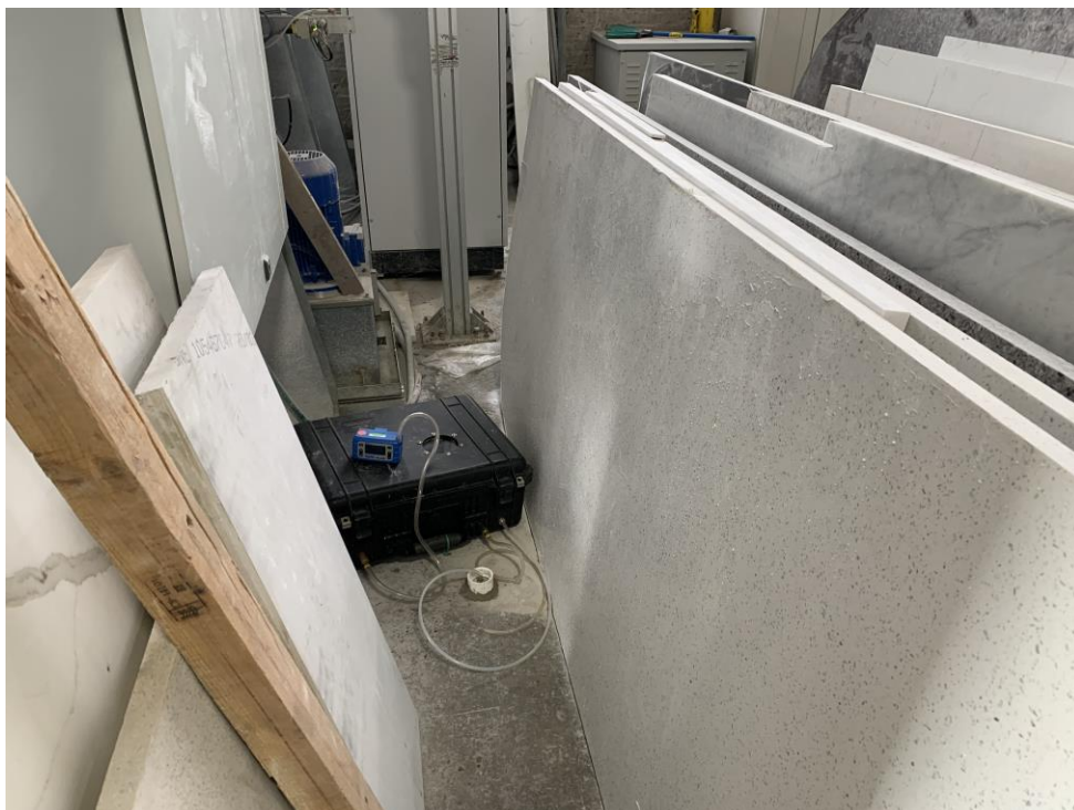
Photo 10: View of vacuum chamber setup at sub-slab soil vapor screening point ACME-SSVS-40, facing west (12/23/2020)
