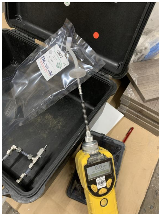
Photo 14: View of Tedlar bag screening at sub-slab soil vapor screening point ACME-SSVS-26B (12/23/2020)
