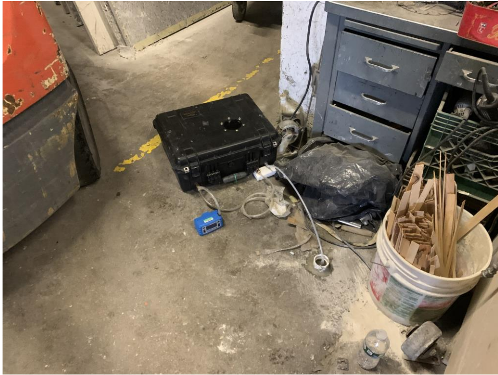
Photo 7: View of vacuum chamber setup at sub-slab soil vapor screening point ACME-SSVS-48, facing southeast (12/21/2020)
