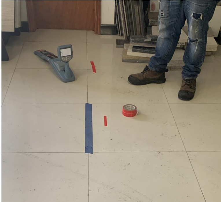
Photo 3: View of NOVA marking out underground utility lines using an electromagnetic detector and tape, facing west (12/18/2020)
