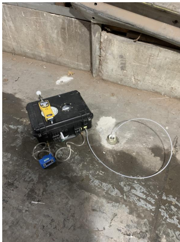
Photo 6: View of vacuum chamber setup at sub-slab soil vapor screening point ACME-SSVS-02, facing west (12/21/2020)
