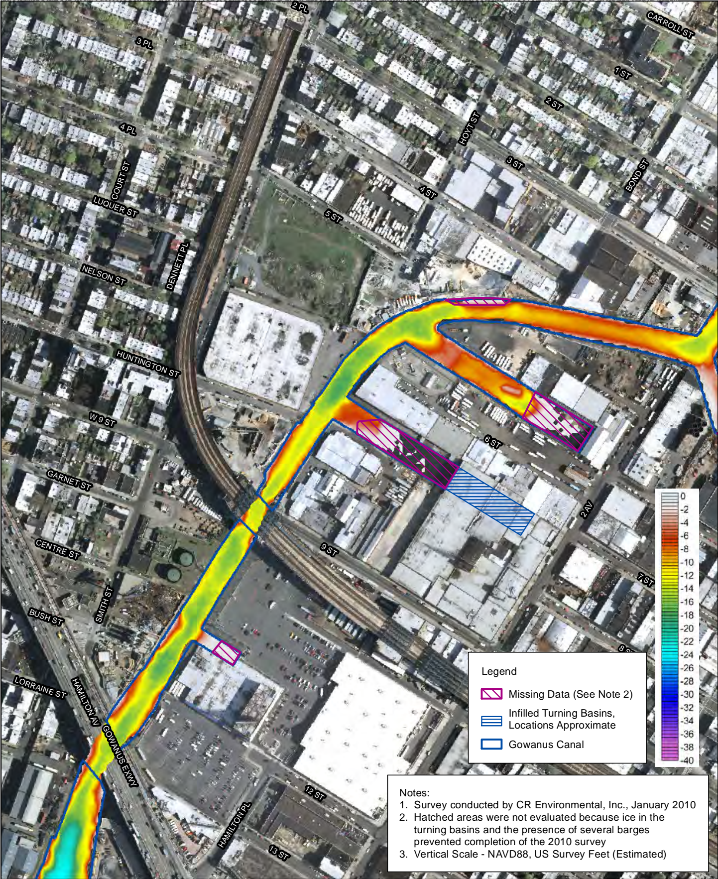
FIGURE 1-5b Bathymetric Map of Gowanus Canal Middle Canal Gowanus Canal Feasibility Study Brooklyn, New York
