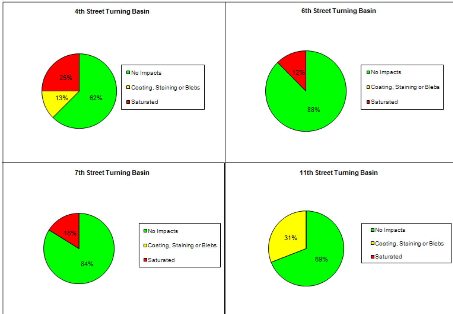
FIGURE 4b Turning Basin Soft Sediment NAPL Impacts Gowanus Canal Feasibility Study Brooklyn, New York
