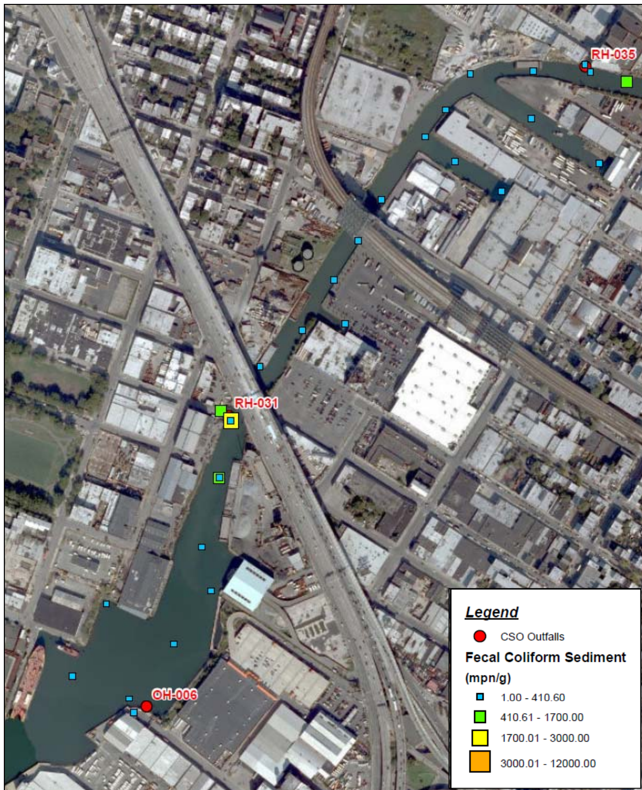
FIGURE 14b Fecal Coliform Distribution in Surface Sediment – Lower Canal Gowanus Canal, Brooklyn, New York
