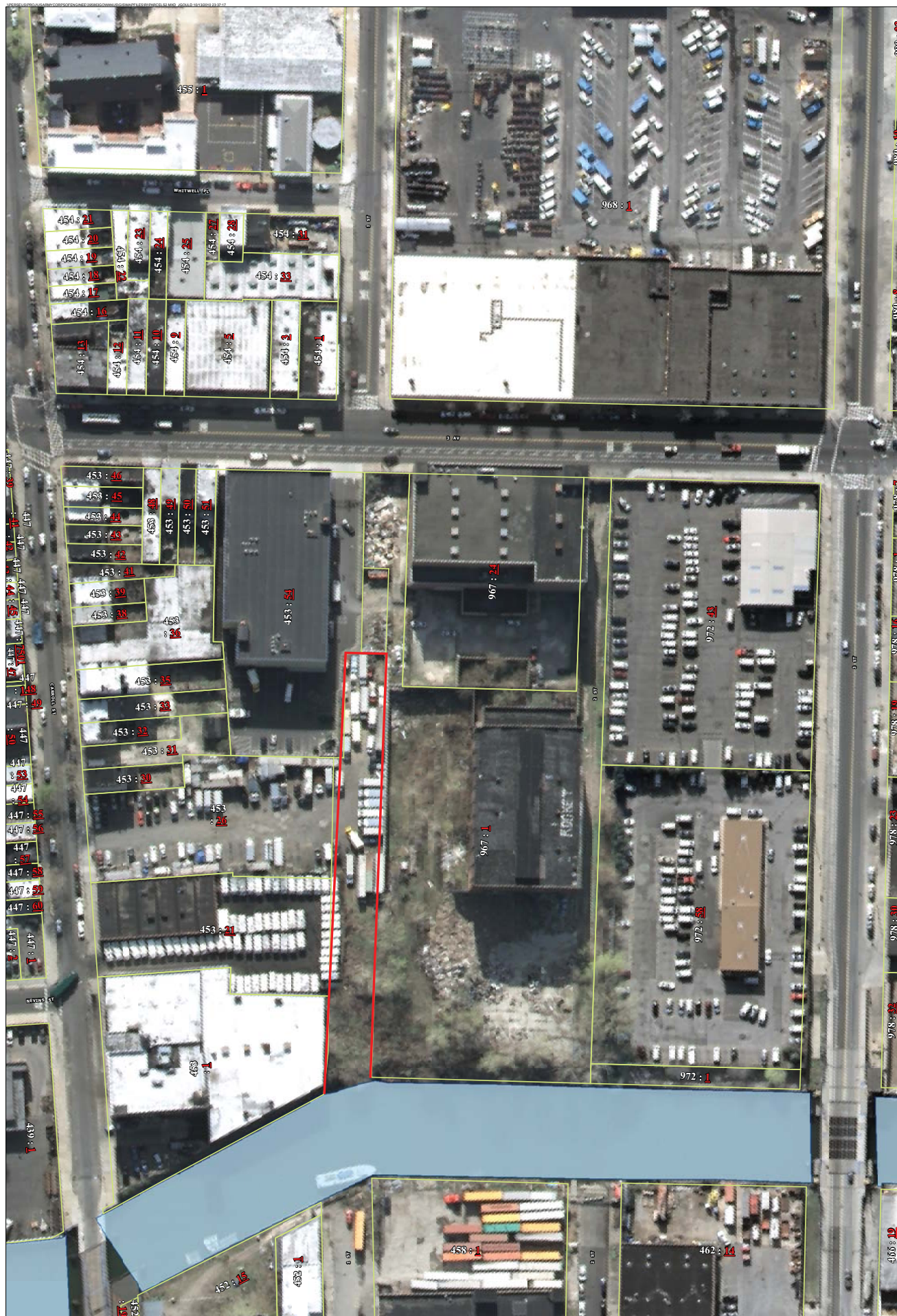
Figure 1 Limits of Considered 1 st Street Turning Basin Excavation Gowanus Canal RI/FS Brooklyn, New York
