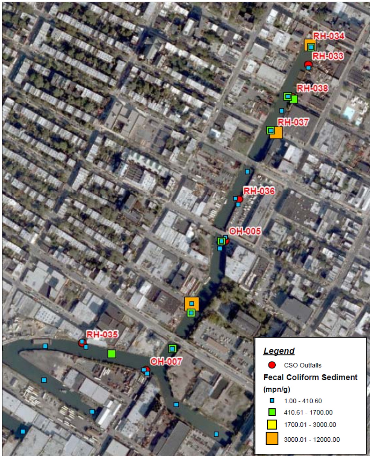
FIGURE 14a Fecal Coliform Distribution in Surface Sediment – Upper Canal Gowanus Canal, Brooklyn, New York
