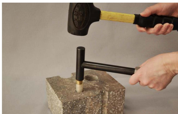
Figure 2. Installing the VAPOR PIN®
