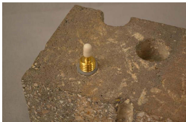
Figure 3. Installed VAPOR PIN®
