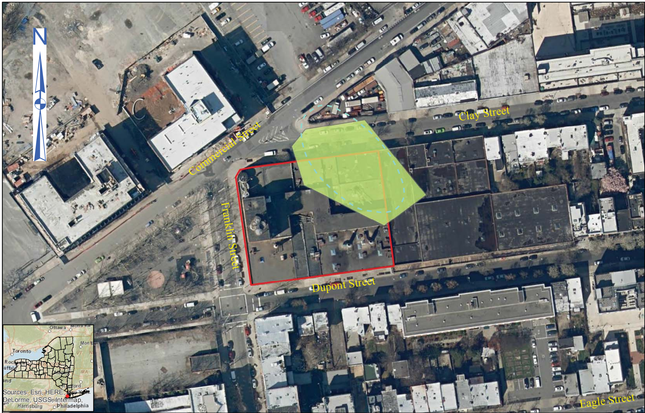
Figure 8 - AS/SVE Treatment Area
