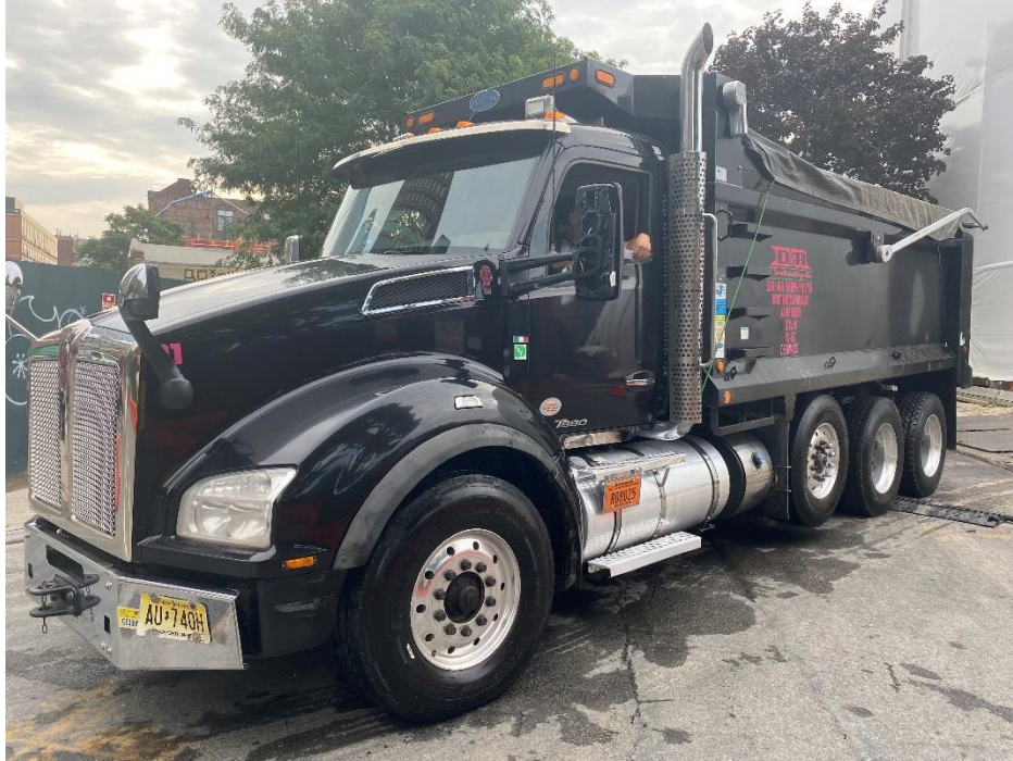
Photo 1: View of covered truck exiting the site containing soil from 0 to 6 ft bgs.
