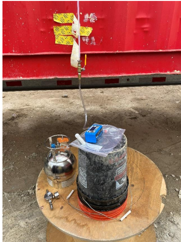
Photo 1: View of air handler unit sampling equipment set up.
