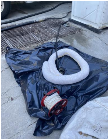
Photo 2: View of spill containment setup, interface probe meter and vac truck flexible hose inserted into RW-25.
