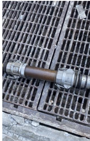
Photo 5: View of LNAPL extraction passing through transparent pipe section of vac truck flexible hose.
