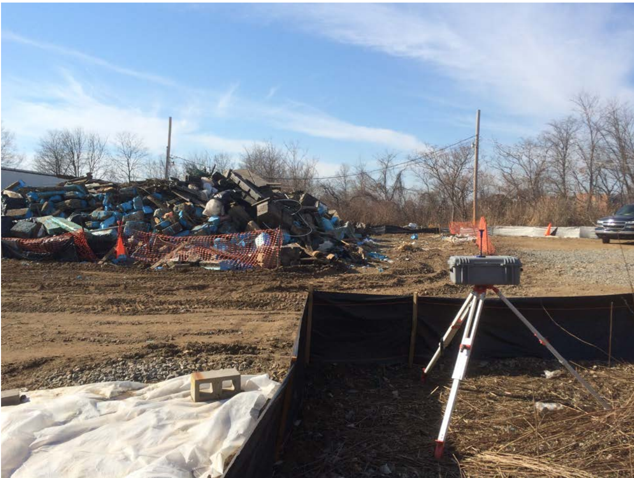
Photo 1: South Dust Trak and Waste Dock Material NW
