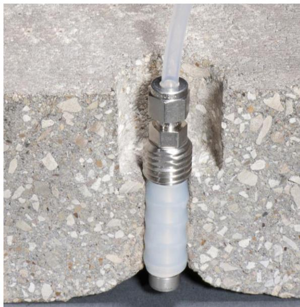
Figure 6. FLX-VP with Swagelok® connection
