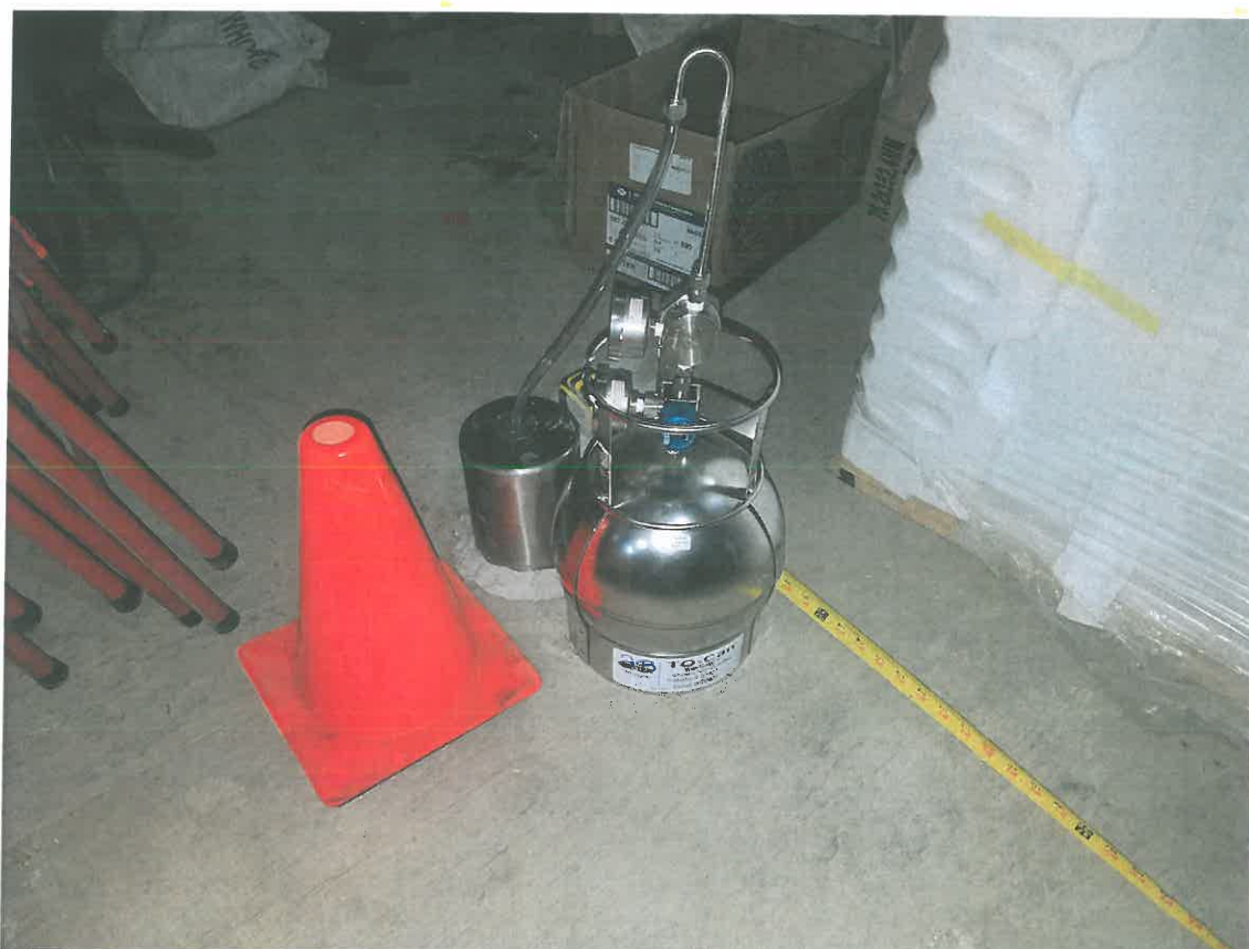
6. View of location of sub slab soil vapor sample (SS2) in ground floor slab.
