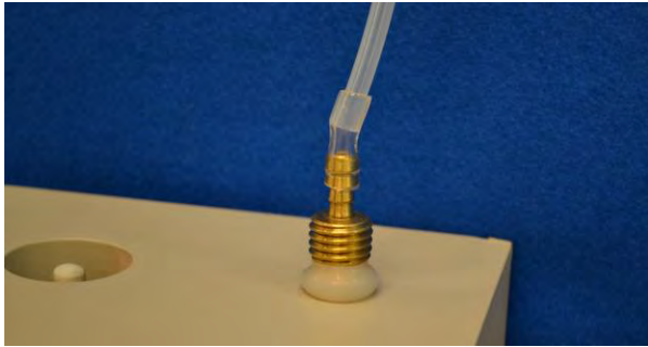
Figure 5. VAPOR PIN® sample connection
