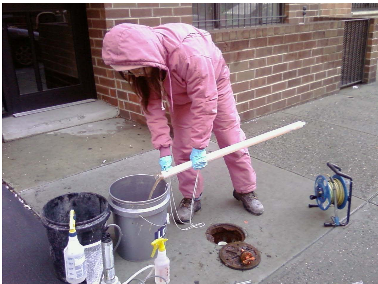
Bailing and collecting groundwater samples at MW-6.
