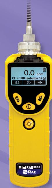
The MiniRAE 3000 is a comprehensive handheld VOC (Volatile Organic Compound) monitor that uses a third-generation patented PID technology to accurately measure more ionizable chemicals than any other device on the market. It provides full-range measurement from 0 to 15,000 ppm of VOCs.
