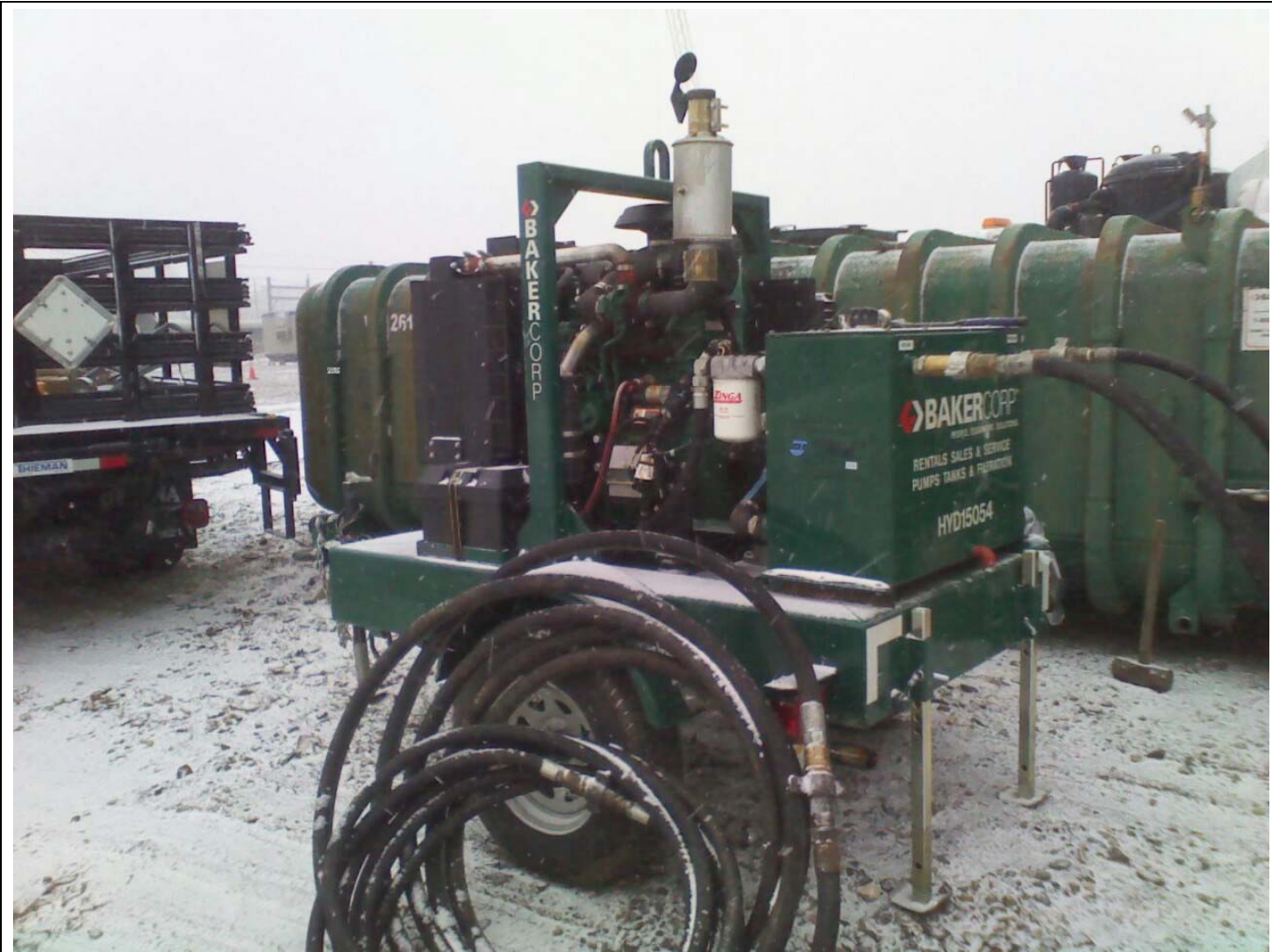
Photo 3. View of hydraulic pump during water by-pass activities.
