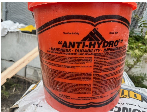
Anti-Hydro concrete admixture was used to boost workability and stability in the wet environment.
