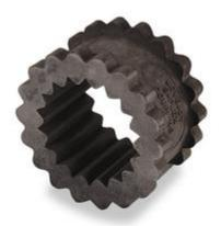
Shaft Coupling Insert, JE Insert Type, 5J Body Style, Rated Torque 240 In-Lb, Max RPM 7600, One-piece Solid EPDM Rubber Insert Material
