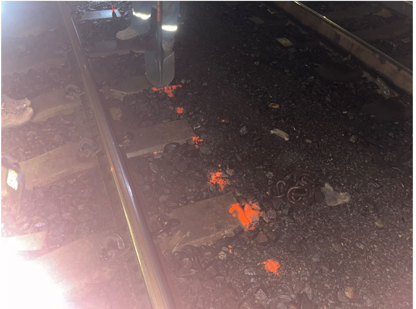
Photo 1: View facing north, MEGA surveying points where samples are to be taken.
