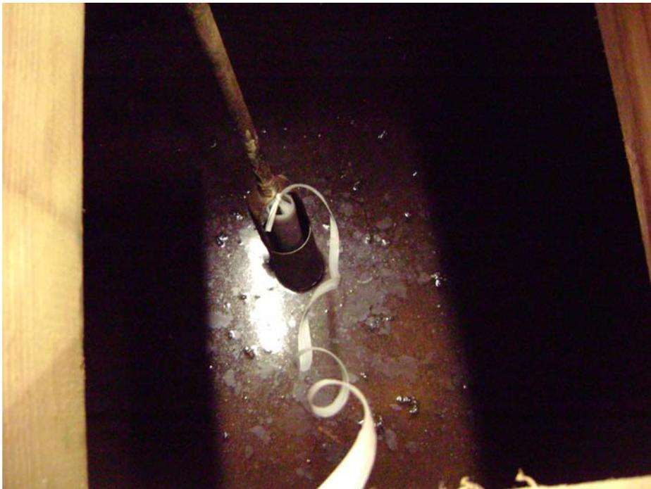
**Photo #4:** Collecting water sample from bottom of Vault with bailer and hand auger for assistance. Sheen visible on water.
