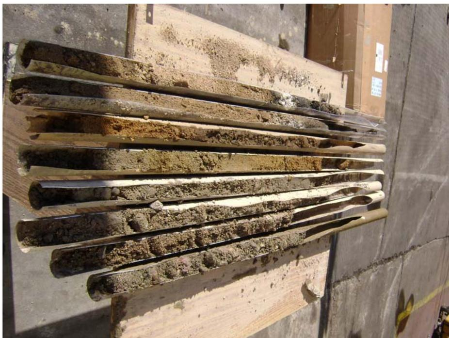
Photo #17: MW14 Soil Borings.
