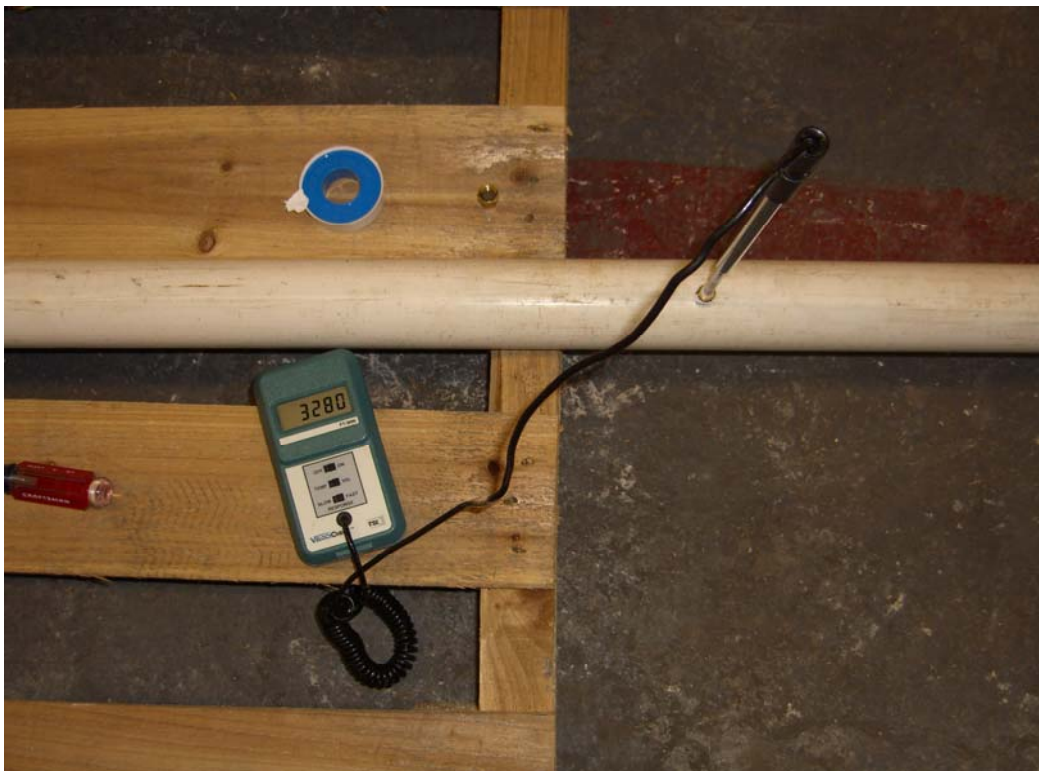
Photo 8: Thermal Anemometer Velocity Measurement
