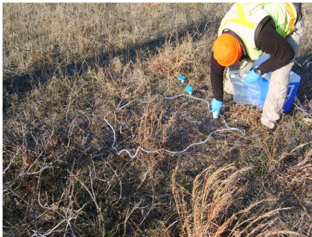
Photo E.1 – 7-point wheel sampling set-up.
