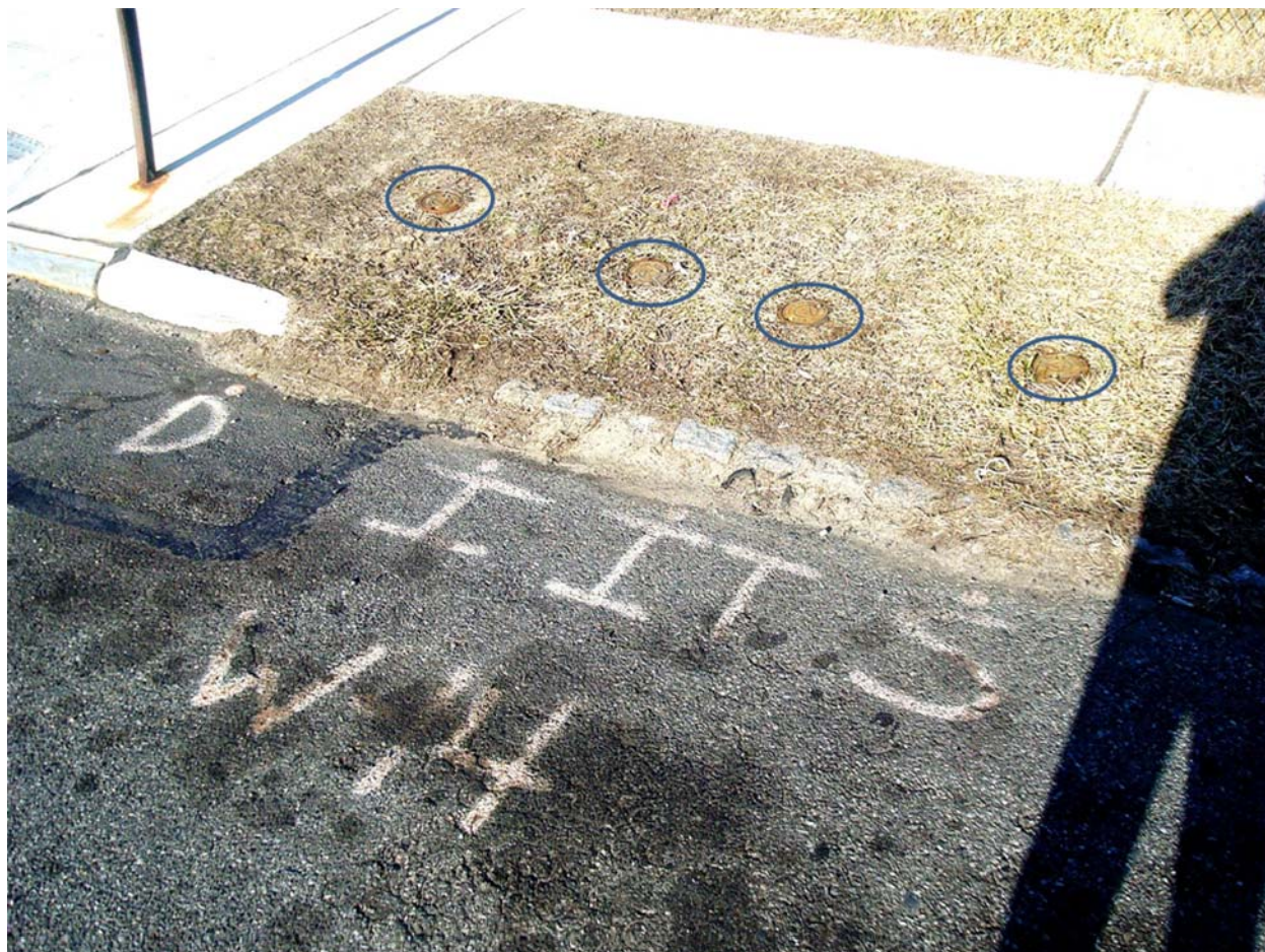
Figure 6-3: Typical Monitoring Well Cluster
