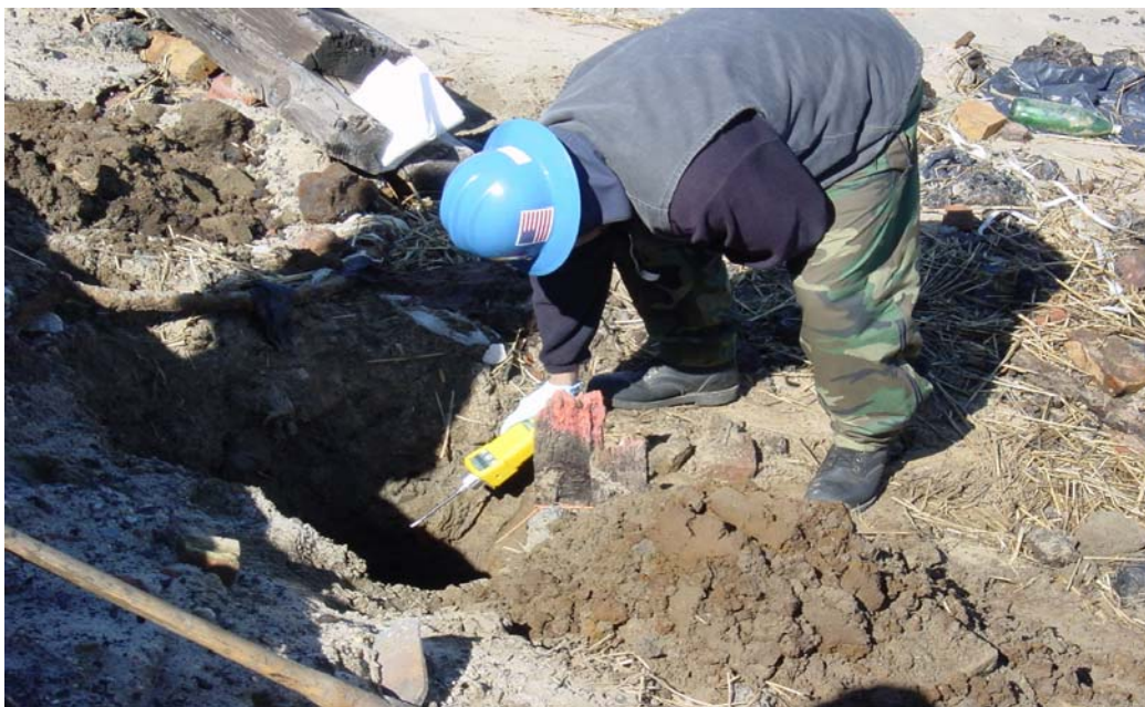
Soil from the excavation was screened with a PID. This was one of the methods used to determine if the soil required disposal.
