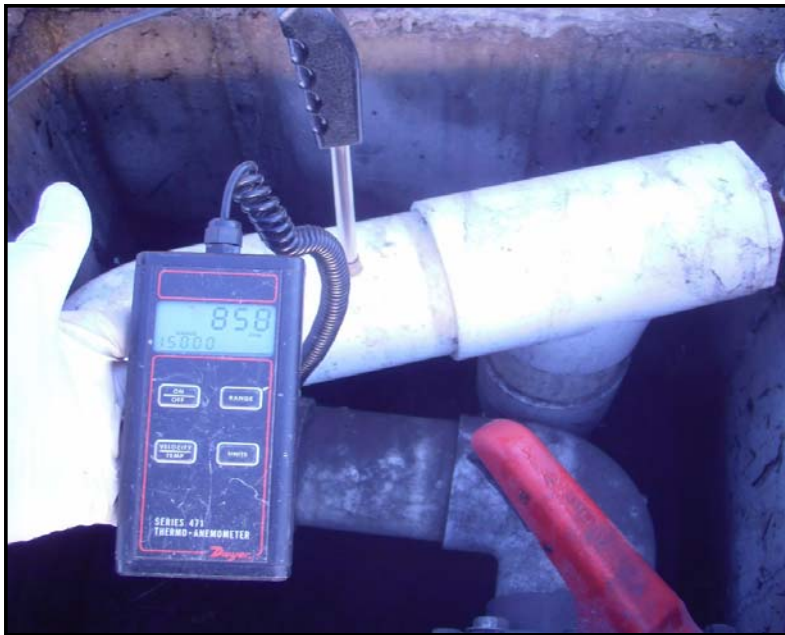
Picture 014.jpg - Velocity measurements were collected from the well heads of the GWTT system.
