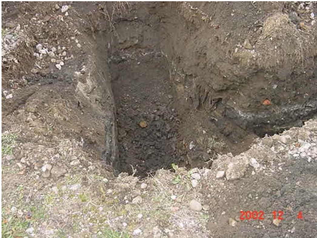
Test Trench Corner Showing Ash and Cinder Layer
