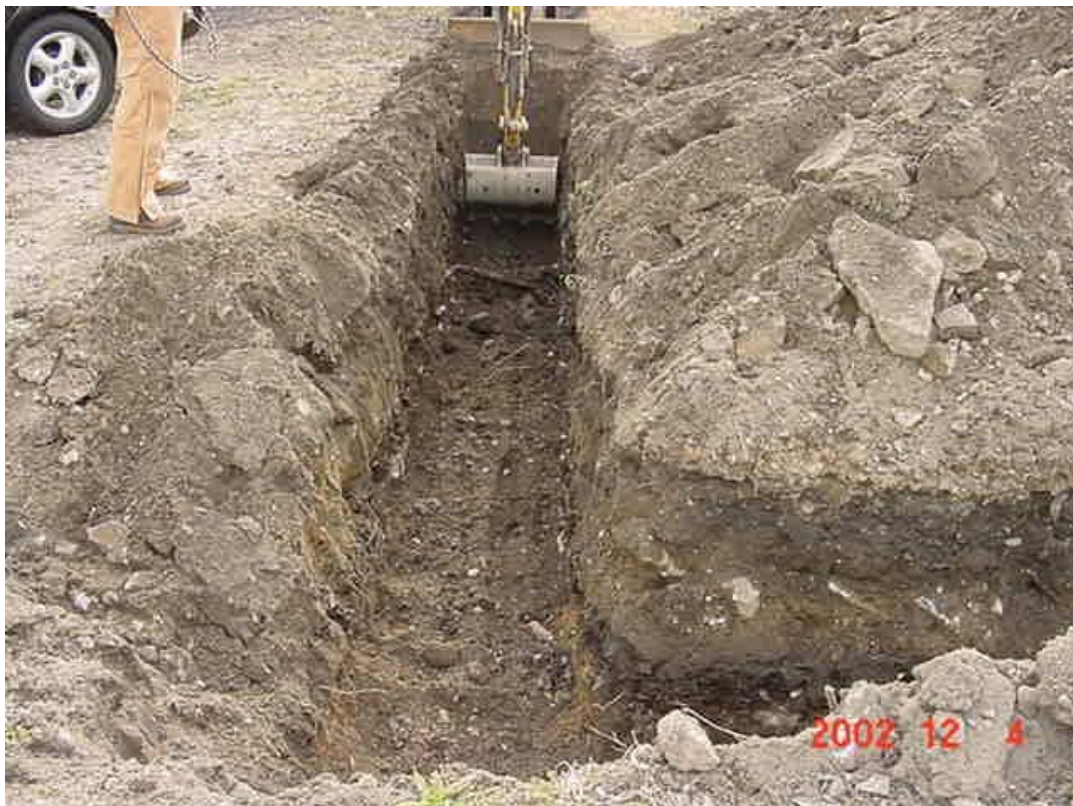
Test Trench Western Branch Showing Ash and Cinder Layer
