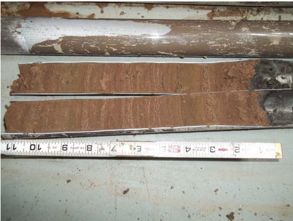
Example of Native Soils Found at Depth in Soil Borings (SB-13, 24 ft bgs)
