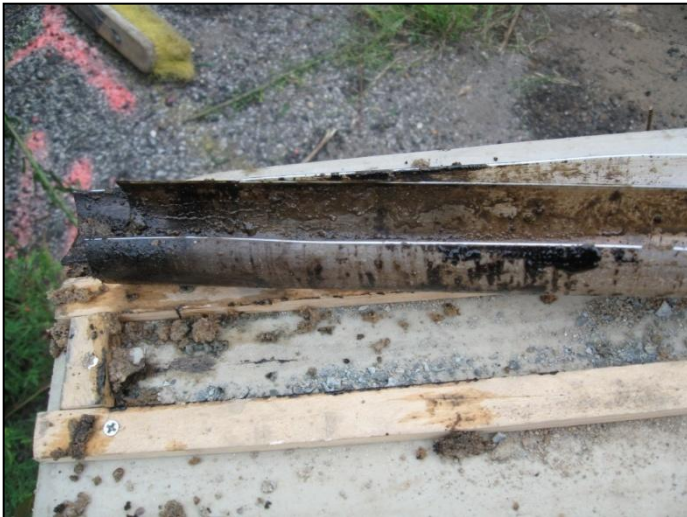
Photograph 7: Soil Boring SB-7 (5-6') – empty liner with suspect petroleum contamination.
