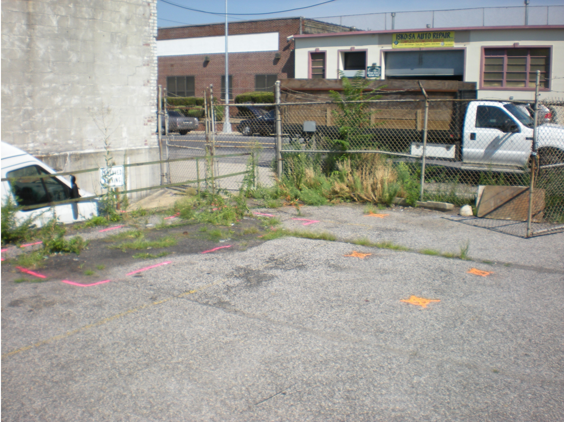
Figure 1 – Metallic anomaly consistent with an UST designated with pink paint. Proposed boring locations are marked in orange.
