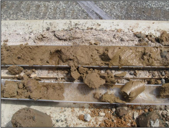
Photograph 5: Silt and sand observed in SB-5. Typical in borings throughout project site.
