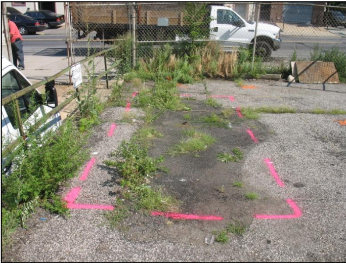
Photograph 1: Underground storage tank locations as identified during geophysical survey (in pink spray paint).
