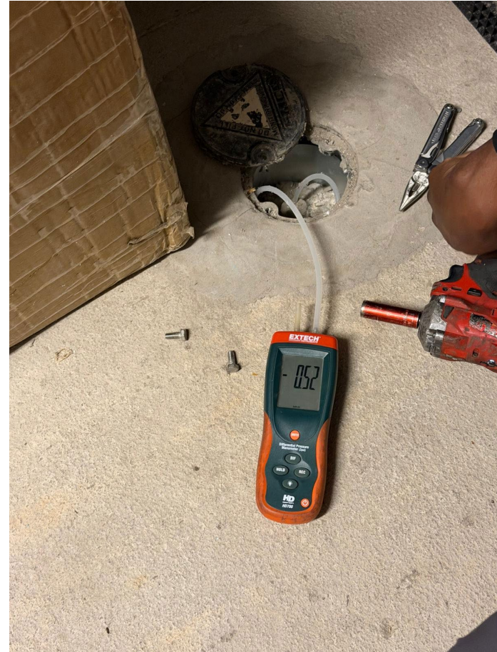
Vacuum measurement at Probe #4
