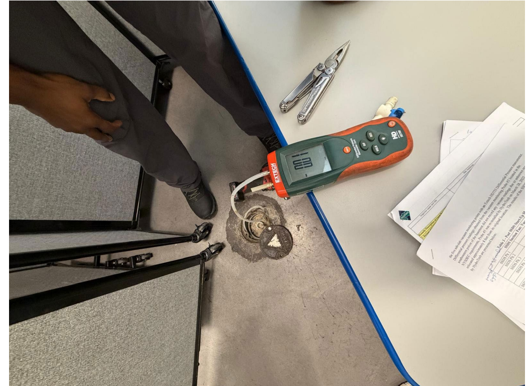
Vacuum measurement at Probe #2
