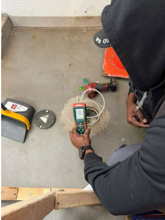
Vacuum measurement at Probe #1
