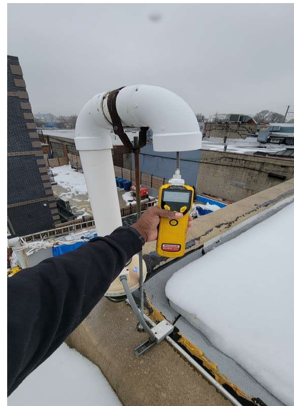
Organic vapor measurement at SVE effluent
