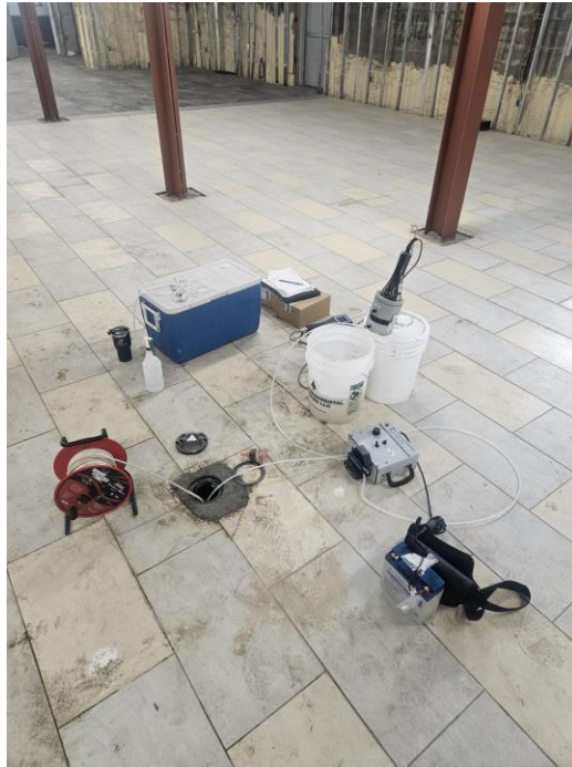
Photo 1: View of groundwater sampling at MW-17, facing northeast.
