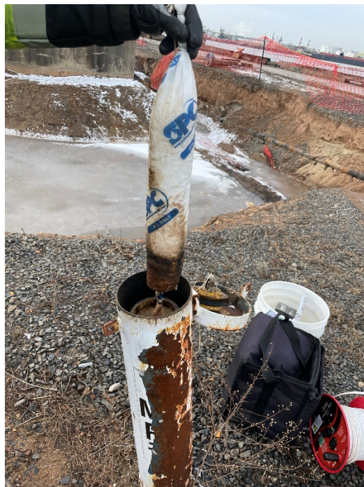
Photo 2: Check of sock in TMP-1 prior to gauging.
