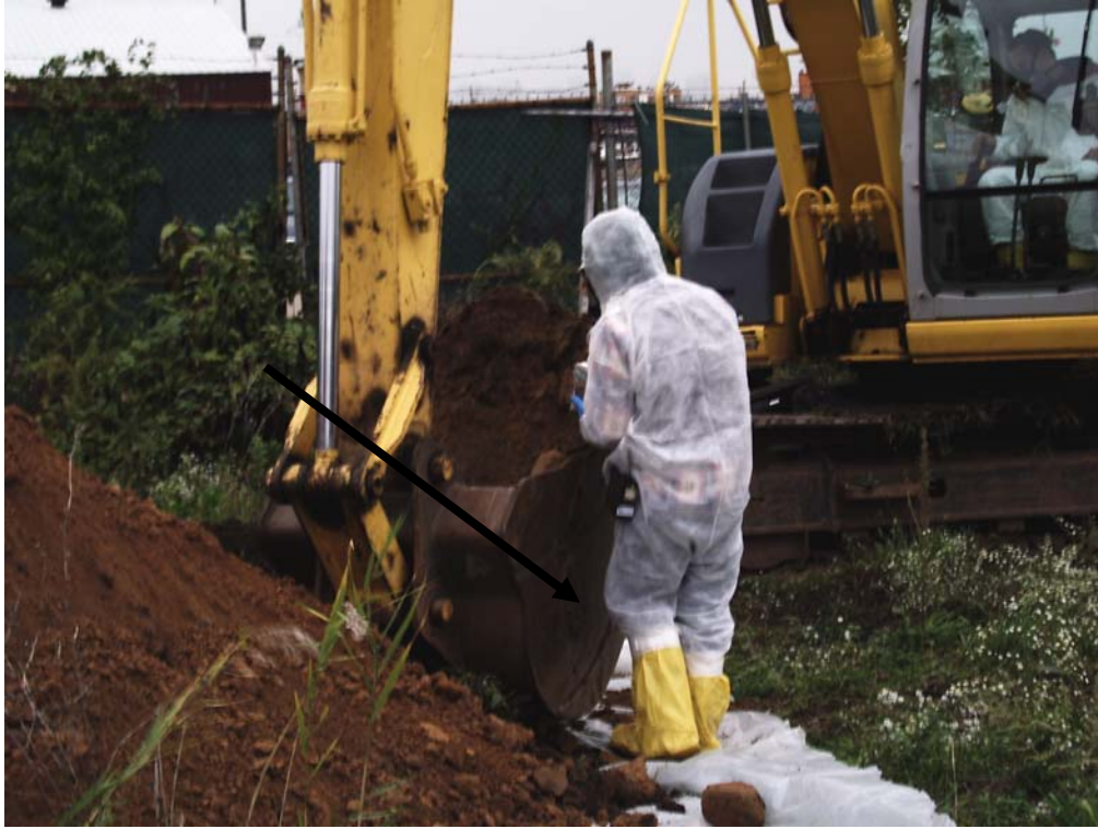
Photograph 3. 4 October 2010. Sampling 6-7 ft depth interval from excavator bucket at Test Pit ZA-1.
