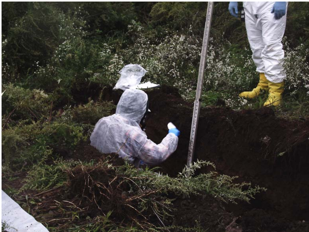
Photograph 2. 4 October 2010. Collecting soil samples from 0-1, 1-2, 2-3, and 3-4 ft depth intervals of Test pit ZA-1.
