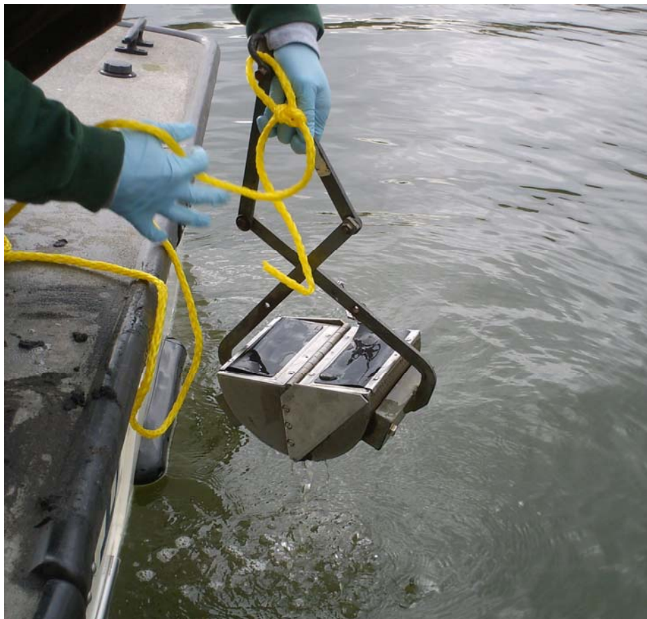
Photograph 9. 19 October 2010. Collecting sediment sample using ponar sampler.
