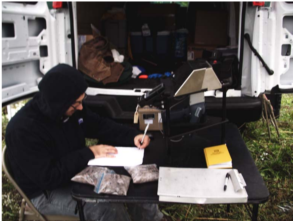
Photograph 4. 6 October 2010. Field portable XRF analytical station.
