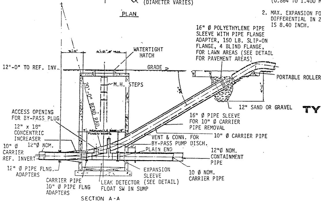
**TYPICAL MANHOLE PLAN & SECTION**
