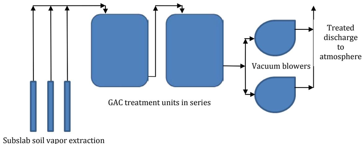
**Exhibit 5.1 – Subslab Vapor Extraction Process Flow Diagram**
