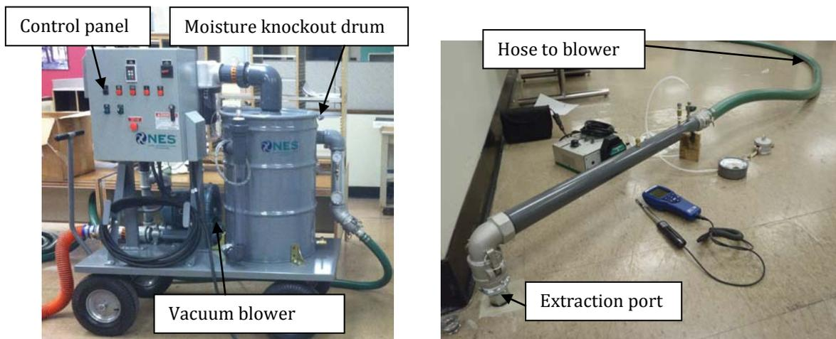
**Exhibit 4.1 – Subslab Extraction Testing Setup.**
