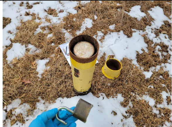
Photo 7 – Typical monitoring well observed in good condition. Well B-3 shown in photograph.
