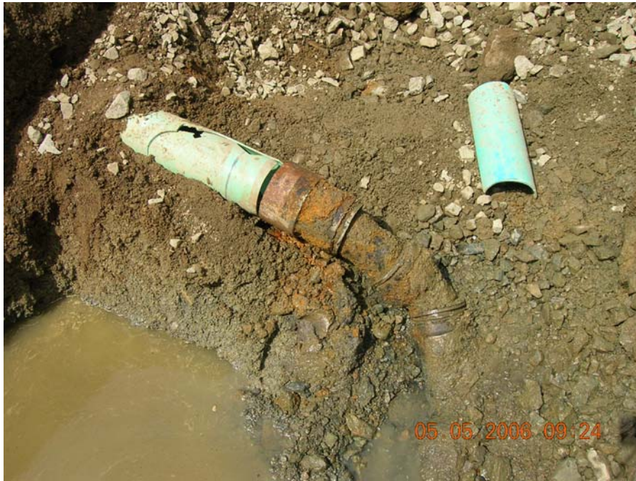
DSCN0293: Failed joint in ISS line from Building 56 area.
