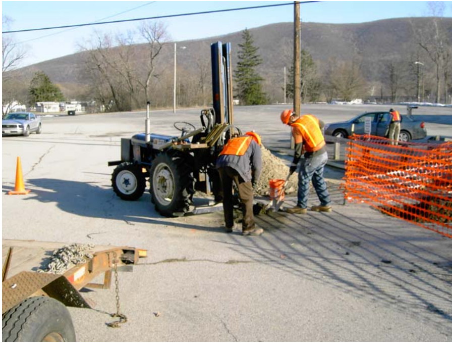
PICT0646: Completing geoprobe borings near Building 31
