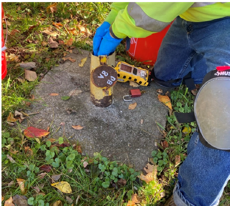
2. Accessing DB-8A for sounding of well.
