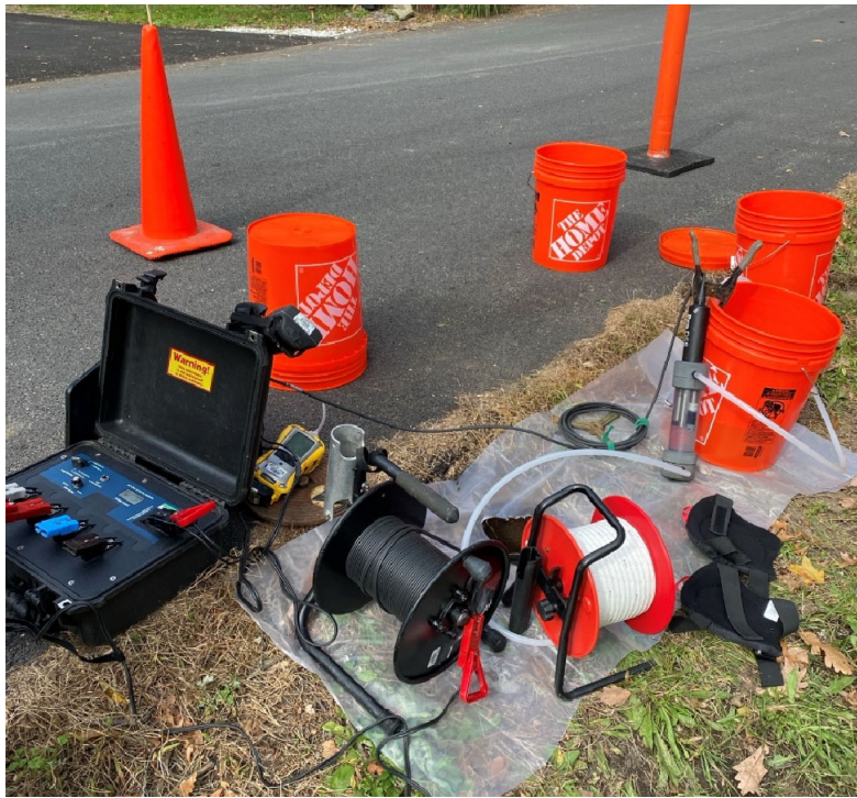
3. Groundwater sampling setup at OS-2.
