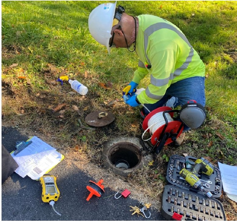
1. Decontamination of interface meter at OS-2.
