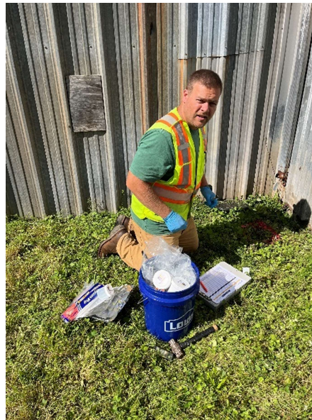
AECOM employee inserting soil vapor sampling media in the ground.
