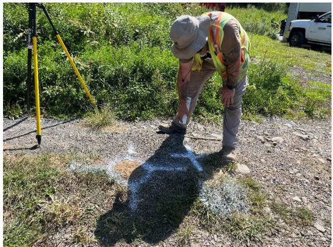
AECOM employee marking soil vapor sample location following installation.
