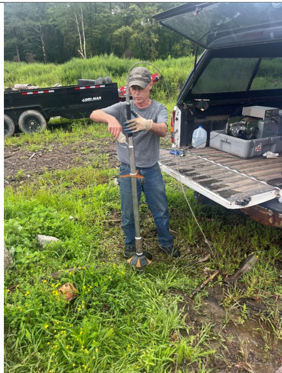
AGS employee rinsing heat pulse probe before inserting it into TW-3.
