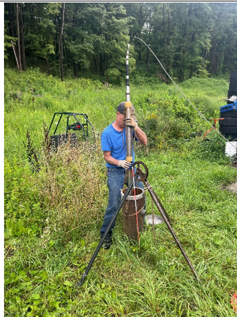
AGS employee inserting probe into TW-2 to conduct acoustic televiewer survey.
