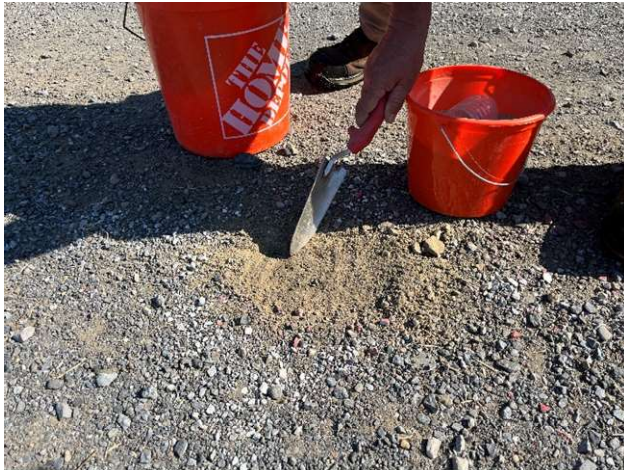
AECOM employee uncovering soil gas passive sampling location.
