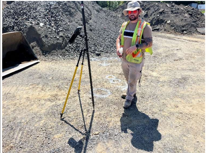
AECOM employee surveying soil vapor sample location.
