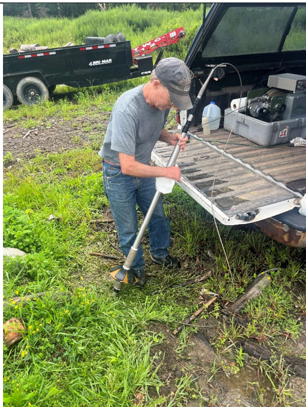
AGS employee wiping off heat pulse probe after completing survey at TW-3.
