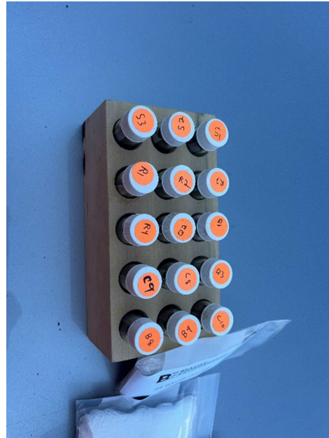
AECOM employee(s) capped soil gas samples with solid caps and labeled them using a ballpoint pen.
