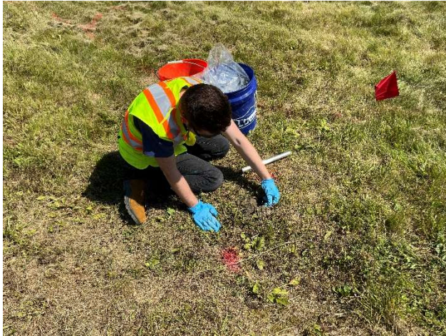
AECOM employee installing soil vapor sample media.
