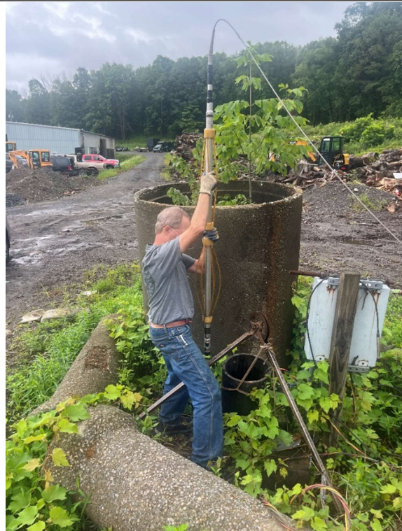
AGS inserting optical televiewer into TW-3.
