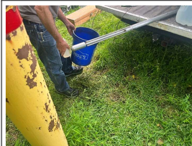
AGS employee decontaminating three-armed caliper.
