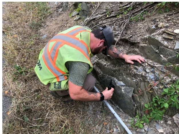
Photo 7 – South – AECOM measuring dip of shale/greywacke interface.
