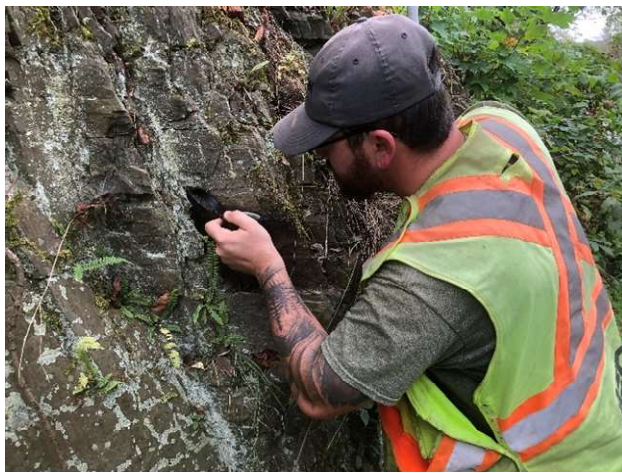
Photo 5 – Southwest – AECOM measuring strike of bedding plane in outcrop #4.
