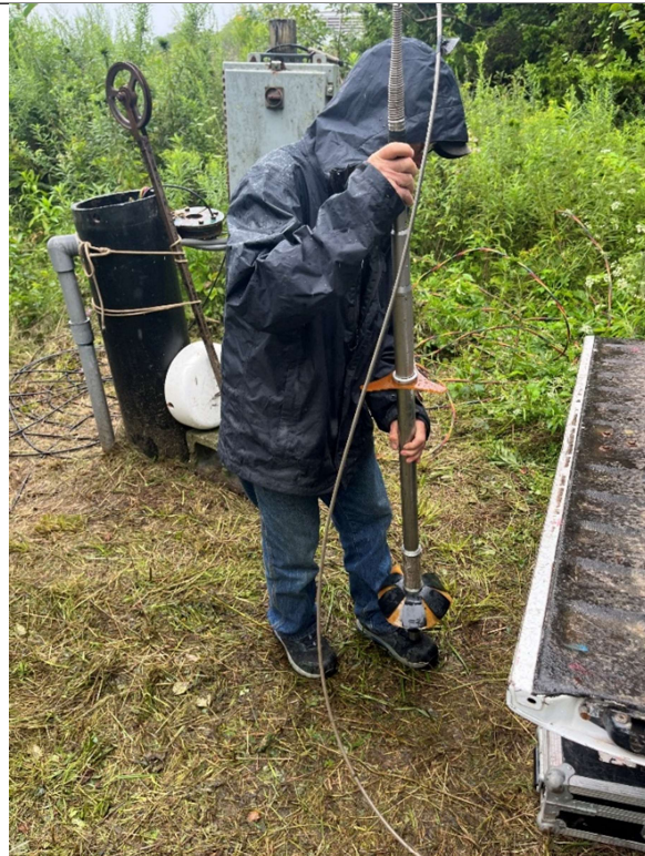
AGS employee removing heat pulse probe from TW-1.
