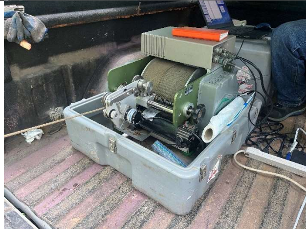
Reel utilized for controlled ascent/descent of probes into wells.
