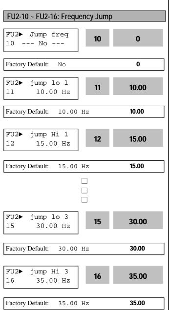
To prevent undesirable resonance and vibration on the structure of the machine, this function locks out the potential resonance frequency from occurring. Three different jump frequency ranges may be set. This avoidance of frequencies does not occur during accelerating or decelerating. It only occurs during continuous operation.
