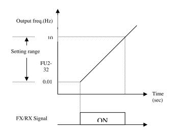
Note: Motor starts running at 5Hz when FU2-32 is set to 5Hz.
