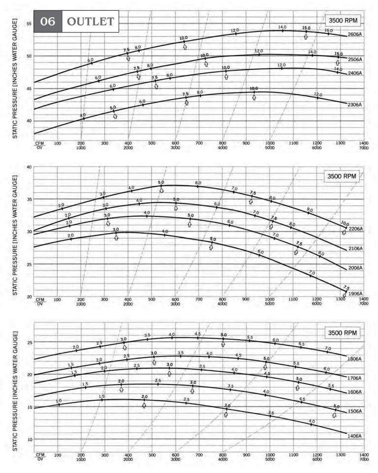
Performance shown is installation Type B: Free inlet, Ducted outlet. Power rating (BHP) does not include drive losses. Performance ratings do not include the effects of appurtenances in airstream.
