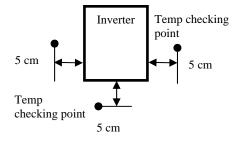
4) The inverter will be very hot during operation. Install it on a non-combustible surface.
