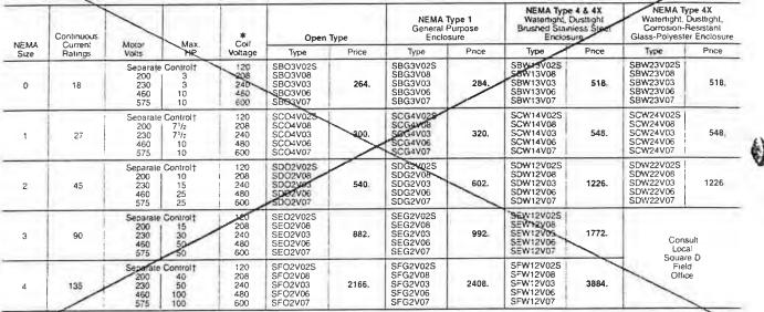
120 Volt Polyphase starters are wired for separate control. Convoltage code must be specified to order this product. Refer to standard coil voltage codes listed in selection table above or additional standard voltage codes below and insert as show in the How To Order block.
