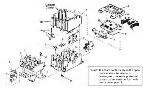
Figure 1 Contactor and Starter Assembly Drawing
