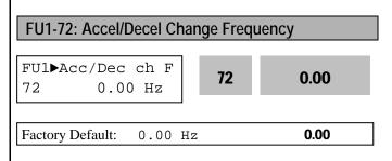
This function is used to change Accel/Decel ramp at a certain frequency. This is useful in textile machine application. For example, when stop command is ON while inverter runs at 100Hz, inverter swiftly decelerates and changes the ramp at this frequency, leading to soft stop.
