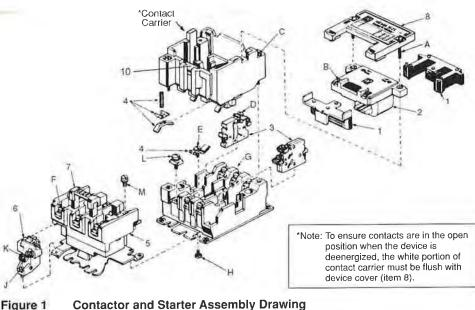
**Contactor and Starter Assembly Drawing**
