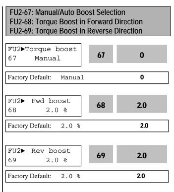
This function is used to increase the starting torque at low speed by increasing the output voltage of the inverter. If the boost value is set too high than required, it may cause the motor flux to saturate, causing over-current trip. Increase the boost value when there is excessive distance between inverter and motor.
