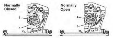
Figure 2 Determining Contact Status
