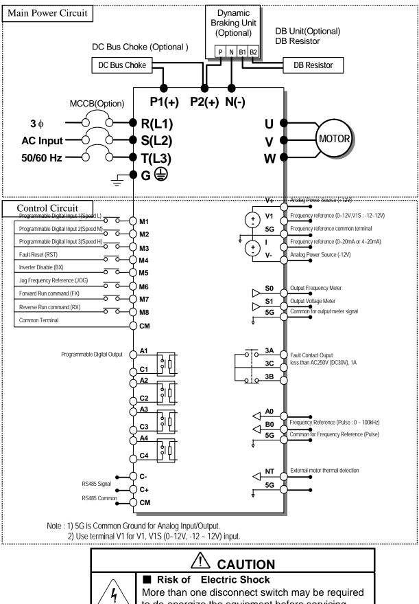
More than one disconnect switch may be required to de-energize the equipment before servicing.
