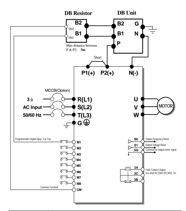
3) Wiring for DB unit and DB resistor (for 5.5~90kW/7.5~125HP inverters)
