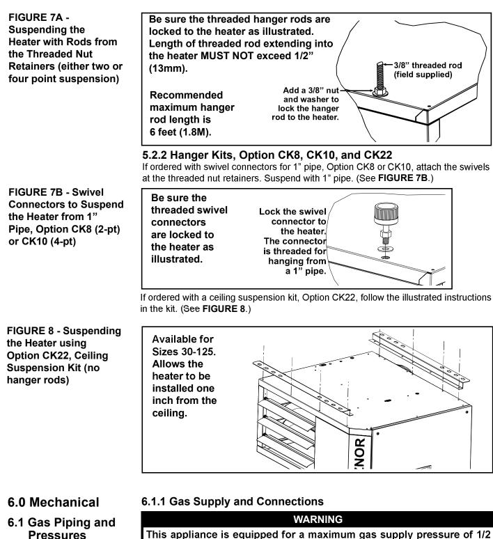
This appliance is equipped for a maximum gas supply pressure of 1/2 psi, 3.5 kPa, or 14 inches water column. Supply pressure greater than 1/2 psi requires installation of an additional lockup-type service regulator external to the unit.
