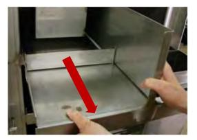
6. Pull the tray straight out and remove it for cleaning. QED can provide specialty tools that make tray removal easier. After cleaning the trays and the other internal surfaces of the stripper, replace everything in reverse order. EDI
