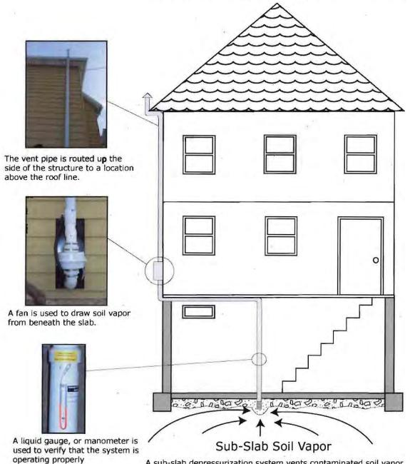
A sub-slab depressurization system vents contaminated soil vapor before it enters a structure. The fan draws vapor from beneath the building outside to the roof line where it is released to the outside air.
