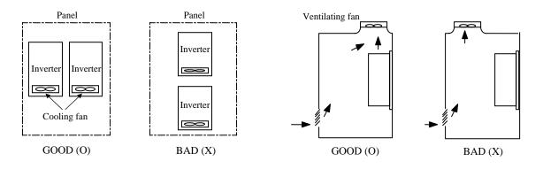
[When installing several inverters in a panel]
