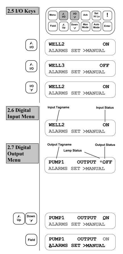
Pressing the I/O Up or I/O Down keys will scroll through the operational I/O points in the system. Data relevant to a particular I/O point will be displayed to right of the point's Tagname.
