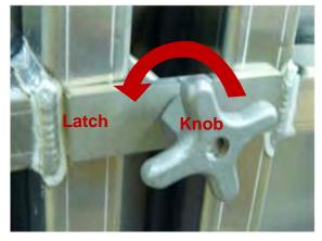
**1.** Loosen the door knobs by turning them counterclockwise.
