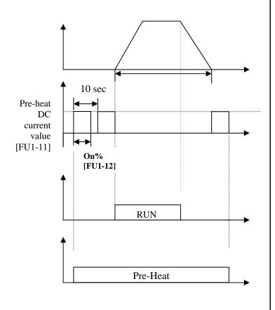
Pre-heat function is activated when FU1-10 [Pre-heat] is set to "Yes", one of the Programmable digital input terminals in I/O-20~27 set to "Pre-heat" and the defined terminal is turned ON. Only active at inverter stop.
