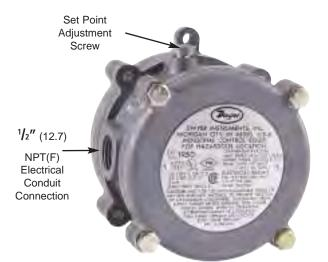
Series 1950 Explosion-Proof Differential Pressure Switches combine the best features of the Dwyer Series 1900 Pressure Switch with an integral explosion-proof and weather-proof housing. Each unit is UL & CSA listed; FM approved for use in Class I, Groups C & D; Class II, Groups E, F, & G; and Class III atmospheres (NEMA 7 & 9). They are totally rain-tight for outdoor installations. Twelve models allow set-points from .03 to 20 inches w.c. and from .5 to 50 psi (3.4 to 345 kPa).
