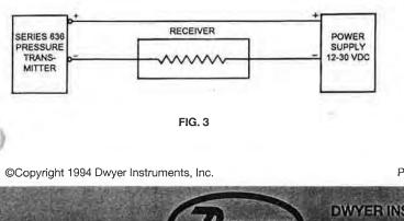
The range of appropriate loop resistance, including the receiver load resistance for the DC power supply being used is limited to that expressed by the graph in Fig. 4.
