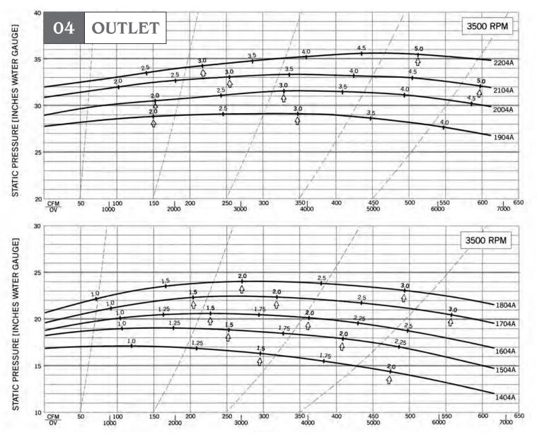
Performance shown is installation Type B: Free inlet, Ducted outlet. Power rating (BHP) does not include drive losses. Performance ratings do not include the effects of appurtenances in airstream.
