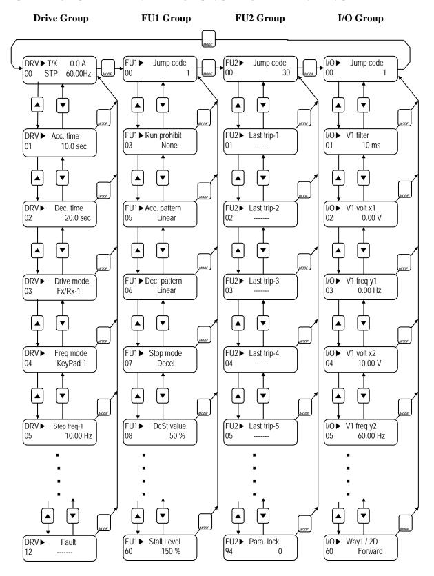
**Note:** This figure shows the group and code navigation through LCD display keypad. It can be different from the actual display due to the group addition or code change.
