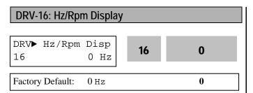
Set this parameter to 0 [Hz] to display frequency, or to 1[Rpm] to display speed.
