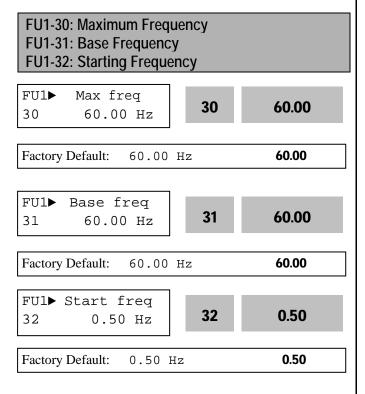
FU1-30 [Maximum Frequency] is the maximum output frequency of the inverter. Make sure this maximum frequency does not exceed the rated speed of the motor.
