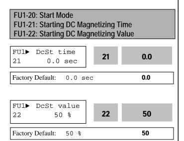
Inverter holds the starting frequency for Starting DC Magnetizing Time. It outputs DC voltage to the motor for FU1-21 [Starting DC Magnetizing Time] with the FU1-22 [Starting DC Magnetizing Value] before accelerating.
