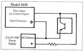
Flow input or control input using open-collector npn transistor with pull-up resistor
