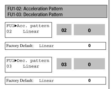
Different combinations of acceleration and deceleration patterns can be selected according to the application.
