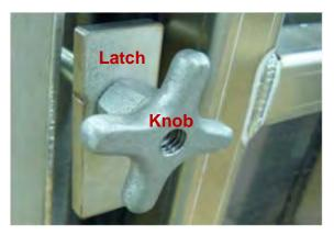
3. Loosen the side knobs until the latches can be rotated to the vertical position. The knobs and latches can be left in place on the two outside door sides. The knobs and latches must be completely removed from all of the door sides in the middle of the stripper. Swing the hinged doors open to gain access to the trays.
