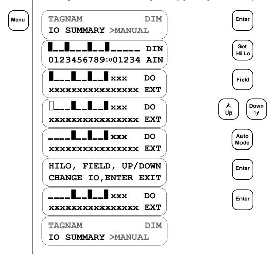
**MODES** Use the Up and Down keys to toggle an Analog Output from Manual control to PID control or Proportional control, depending on which analog output process is being used. This selection will only appear if an analog output tagname is displayed and the analog output is part of an analog output process.
