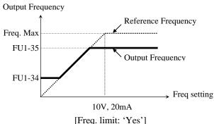
Note: if freq set value is below freq low limit, inverter operates at the low limit.
