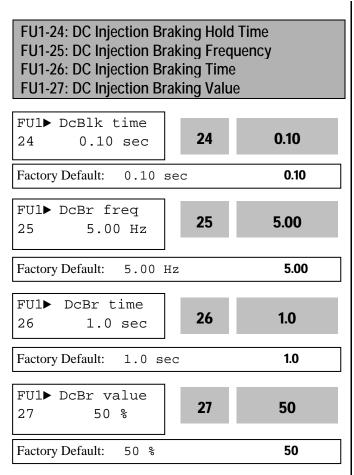
By introducing a DC voltage to the motor windings this function stops the motor immediately. Selecting 'DC-Brake' in FU1-23 activates FU1-24 through FU1-27.
