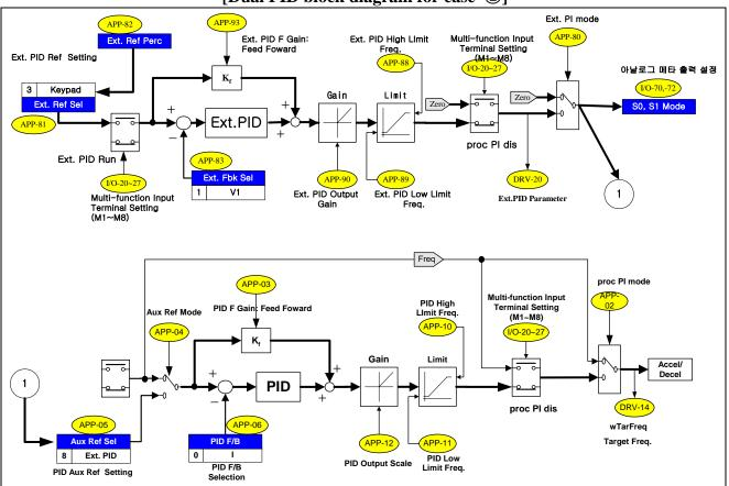
[Dual PID block diagram for case 2]
