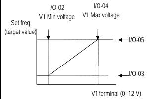
Setting for Bi-polarity and the uni-polarity is the same as the graph above. Set the positive value for Voltage and frequency and negative value is symmetrical of positive setting. The following graph shows the relationship between voltage input and direction command (Positive/Negative).
