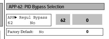
This is used to bypass the PID operation selected in APP-02. Select this code to 'Yes' when using MMC function without PID control. The frequency is determined by actual value (feedback) of control amount instead of PID controller output. The actual value is also used as the Start/Stop reference of Aux. motors.
