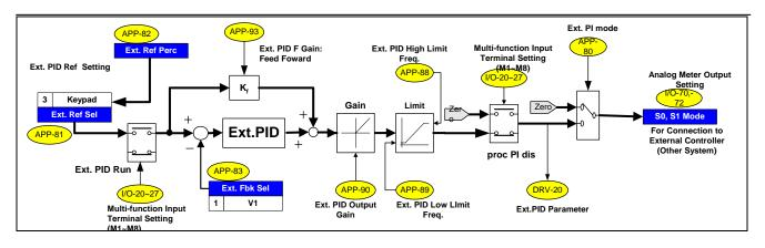
[Dual PID block diagram for case ①]
