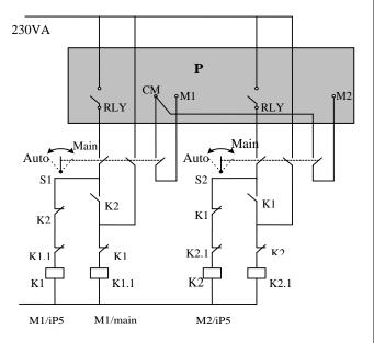
[Sequence Circuit for Inter-Lock Configuration]
