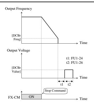
[DC Injection Braking Operation]
