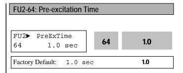
When the operation command (FWD, REV) is issued, the inverter conducts pre-exciting automatically for the time specified by this parameter.
