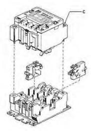
Figure 5 Internal Auxiliary Contacts
