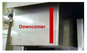
**5.** Remove the trays starting with the top tray and working down. Each downcomer will need to be raised to allow enough clearance to slide the tray out. The downcomer will need to be completely removed on the bottom-most tray. If "seal pots" (shallow black plastic pots) are being used at the base of the downcomers, gently raise the front end of the "seal pot" to pour the water out of it prior to sliding the tray out. Emptying the "seal pots" prevents water from splashing onto personnel.
