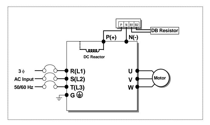
5) For 37~90kW (50~125HP) Built-in DCL Type
