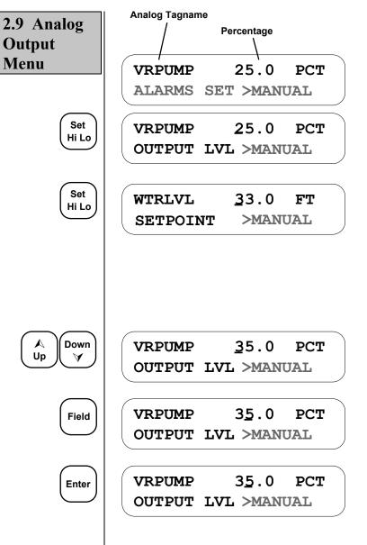
An analog output displayed in the operations screen will be displayed as shown to the left. The percentage of full scale output will be displayed as well.
