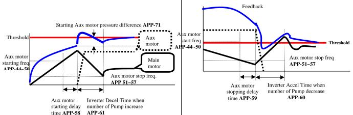
Aux motor active condition: Main motor speed exceeds Aux motor starting frequency (APP-44~50), for the time over APP-58[Aux motor starting delay time], Difference between PID reference and Feedback value exceeds APP-71 [Starting Aux motor pressure difference].
