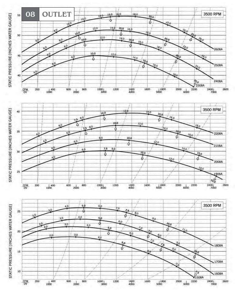
Performance shown is installation Type B: Free inlet, Ducted outlet. Power rating (BHP) does not include drive losses. Performance ratings do not include the effects of appurtenances in airstream.
