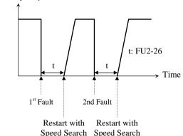
Note: Inverter decreases the retry number by one as a fault occurs. If trip does not occur after restarting for 30 seconds, the inverter increases the retry number by one and maximum number is limited by the value set in FU2-25.
