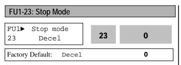
Sets the stopping method for the inverter.
