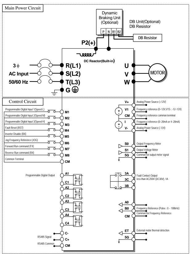
Note : 1) 5G is Common Ground for Analog Meter Output(SO,S1) and External motor thermal detection(ET). 2) Use terminal V1 for V1, V1S (0~12V, -12 ~ 12V) input.
