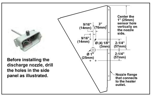
Mount the sensor on the nozzle side.
