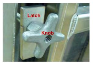
**3.** Loosen the knobs on the sides of the door until the latches can be rotated to the vertical position.
