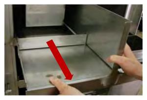
**5.** Pull the tray straight out and remove it for cleaning. QED can provide specialty tools that make tray removal easier. After cleaning the trays and the other internal surfaces of the stripper, replace everything in reverse order.
