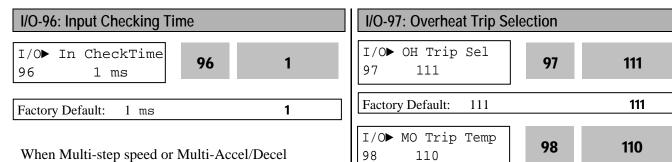
operation is active, inverter determines the input to be valid after the I/O-95 [Input checking time] elapses.
