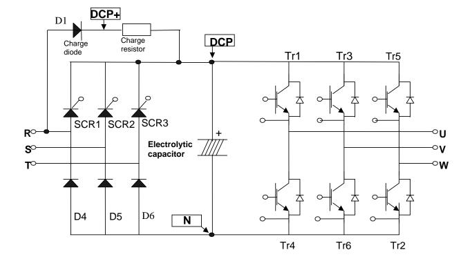
2) Diode module and IGBT module check (37~ 90kW)
