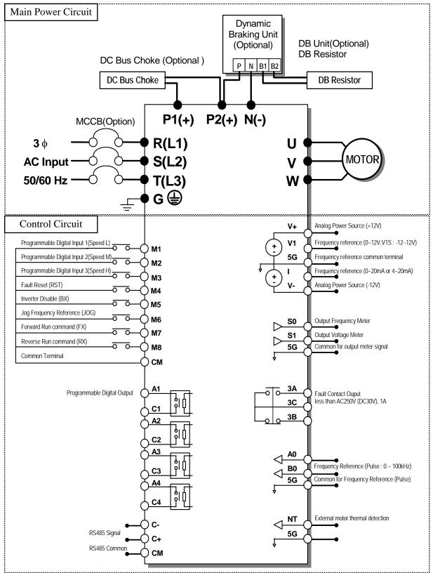
Note : 1) 5G is Common Ground for Analog Input/Output.
