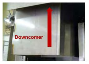
4. Remove the trays starting with the top tray and working down. Each downcomer will need to be raised to allow enough clearance to slide the tray out. The downcomer will need to be completely removed on the bottom-most tray. If "seal pots" (shallow black plastic pots) are being used at the base of the downcomers, gently raise the front end of the "seal pot" to pour the water out of it prior to sliding the tray out. Emptying the "seal pots" prevents water from splashing onto personnel.
