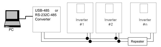
\* REPEATER is not a required item but helps communication in long-distance communication or high noise environment.
