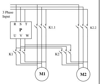
[Wiring Diagram for Inter-Lock Configuration]
