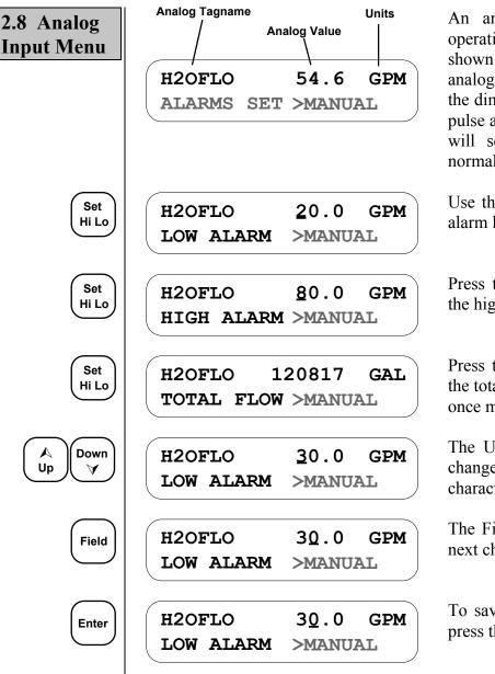
An analog input displayed in the operations screen will be displayed as shown to the left. The value of the analog input will be shown along with the dimensional units. In the case of a pulse accumulator (totalizer only), you will see only TOT where units is normally displayed.
