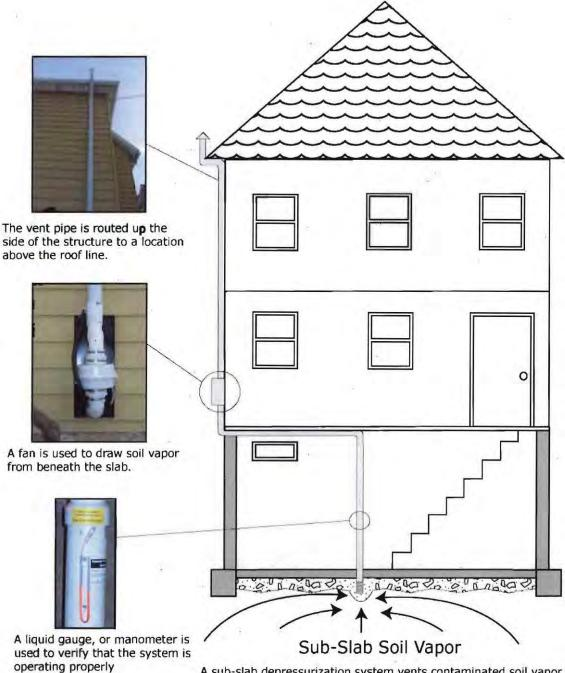
A sub-slab depressurization system vents contaminated soil vapor before it enters a structure. The fan draws vapor from beneath the building outside to the roof line where it is released to the outside air.
