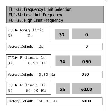
FU1-33 selects the limits the inverter operating frequency. If FU1-33 is set to 'Yes', inverter operates within the upper and lower limit setting. The inverter operates at the upper or the lower limit when the frequency reference is outside the frequency limit range.
