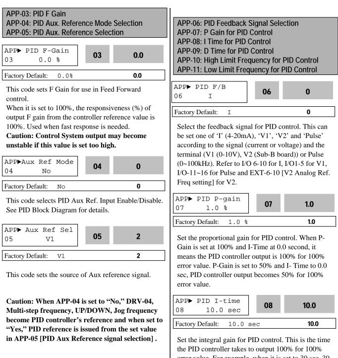
error value. For example, when it is set to 30 sec, 30 sec is taken for PID controller to output 100% for 100% error value. 100% error means feedback value is 0 to the preset reference value.
