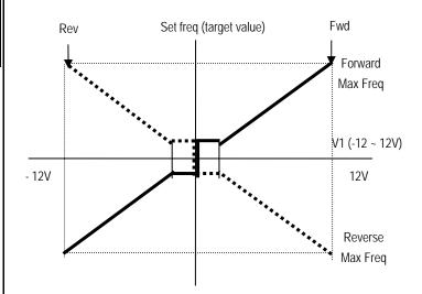
To drive the motor in Forward direction, press FWD key and apply 0-12V voltage as frequency command or press REV key and apply -12~0V voltage as frequency command. To drive the motor in Reverse direction, press FWD key and apply -12~0V or press REV key and apply 0~12V.
