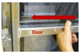
4. Slide the door slightly to the left, turn it on an angle and remove the door by pulling it outward. The knobs may need to be turned to the "X" position to provide enough clearance for door removal.
