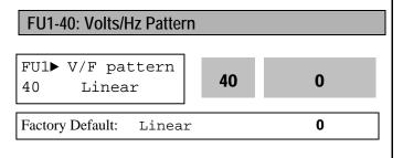
This is the pattern of voltage/frequency ratio. Select the proper V/F pattern according to the load. The motor torque is dependent on this V/F pattern.
