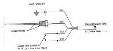
WIRING DIAGRAM FOR MECHANICAL SEAL/HEAT SENSOR Figure 3
