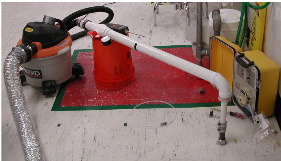
Exhibit 2 - Subslab Extraction Testing Set-Up
