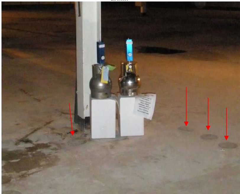
PHOTO #3 – Sample IA0702; located in the Clean Room. Sample is located on an elevated floor near an “acid drain.”
