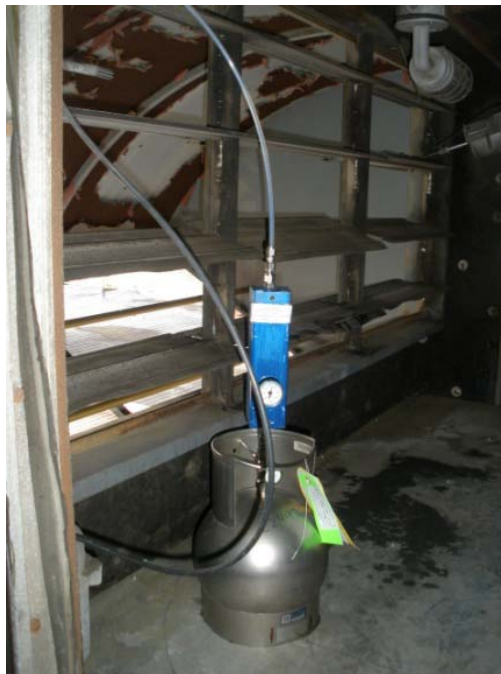
Photos #22: Sample AA-2021, located in the plenum outdoor air intake for AC-32.
